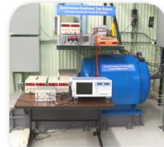
Rotating-based test system for providing reactive power on ckt. 4.
