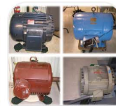
Various sizes (7.5hp - 75 hp) of induction motors in addition to distribution system loads.
