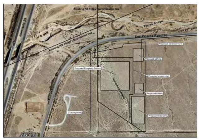
Figure 2-3. Site layout showing proposed facilities.
