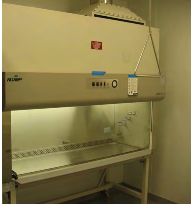
Figure 2-3. Photo of a NUAIR - Class II Type A-2 BSC 12 with Thimble Connection
