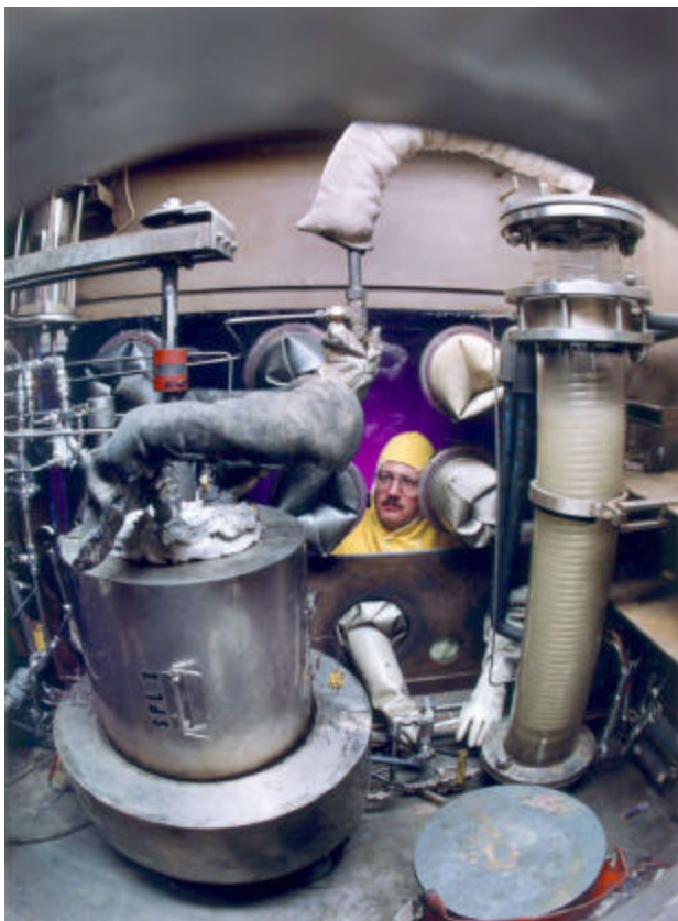
Calciner at PFP
