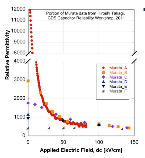
Voltage tuning and dielectric breakdown severely limit stored energy density
