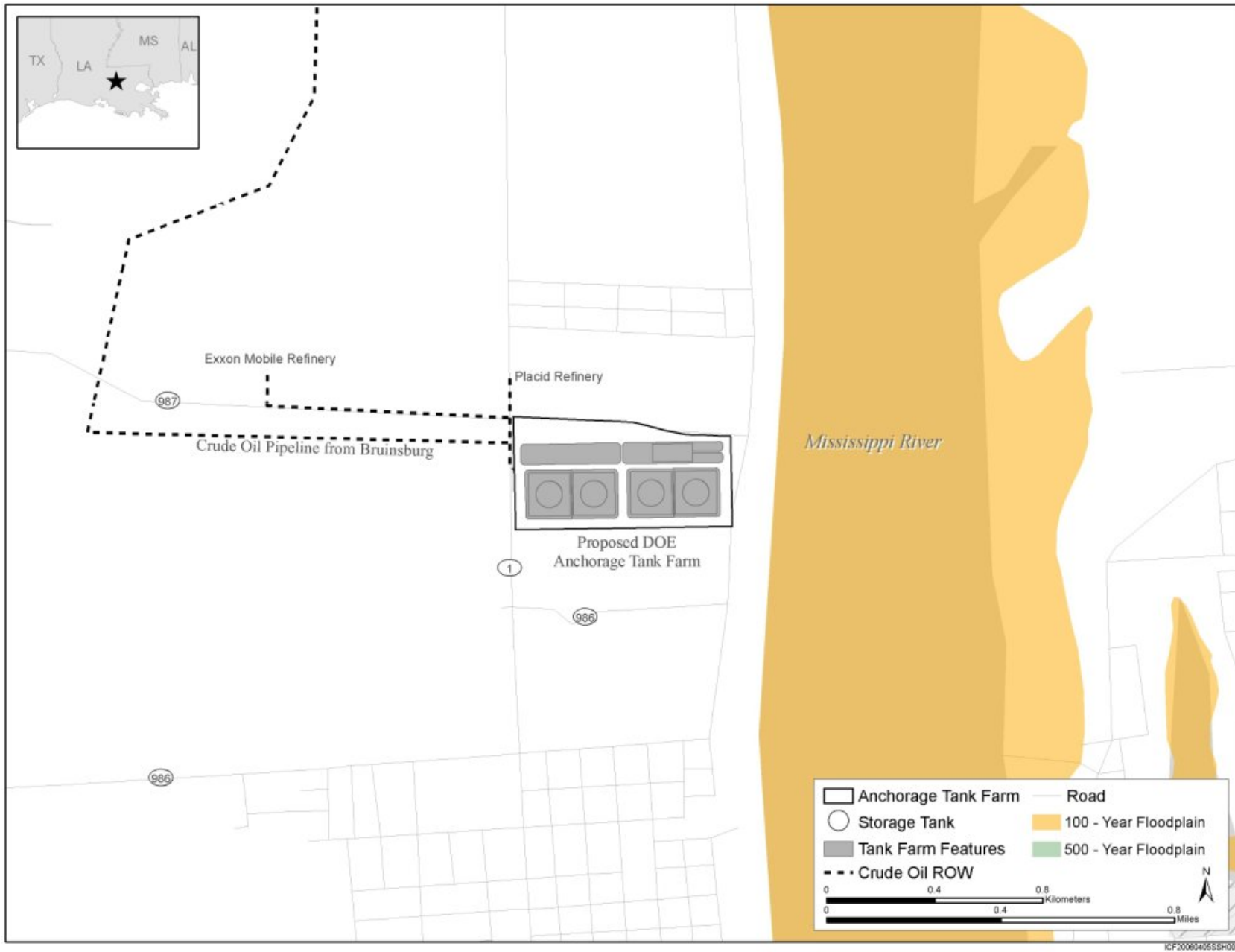
Figure B.6.1-3: Floodplain Map for Anchorage Terminal
