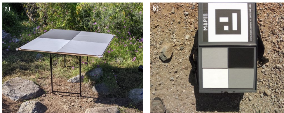
Figure 4. (a) GRP8 and (b) MAPR radiometric calibration panels, each containing multiple grayscale sub-panels corresponding to known traceable reflectance values. The GRP8 panel was located within the UAV's flight path for all UAS missions, while the MAPR panel was imaged with the UAV in-hand at a short distance above the ground before and after each flight.
