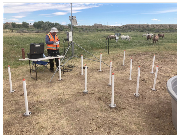
Figure 12. Riverton Site Unsaturated Zone Infiltration Field Tracer Testing with a Downgradient Well Gallery
