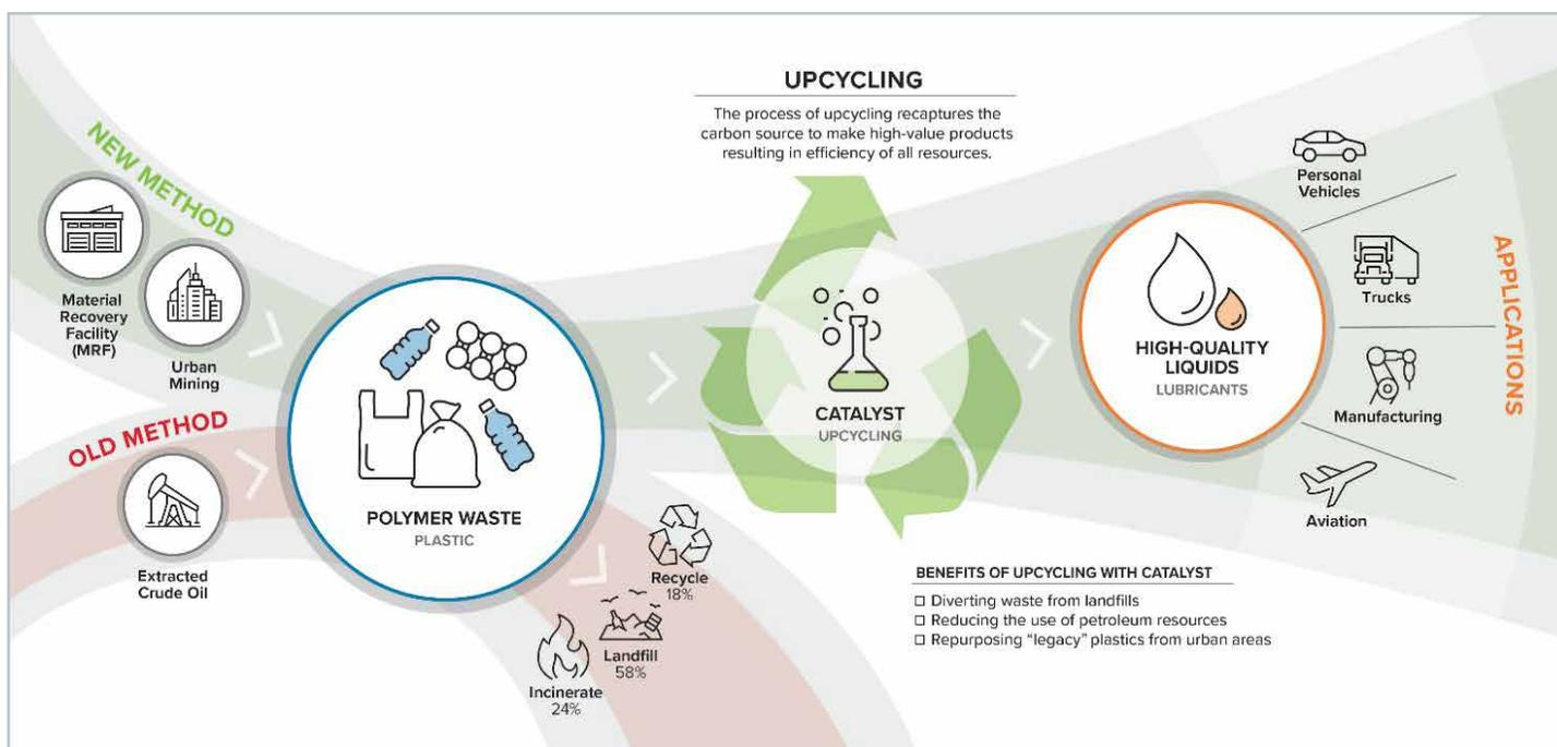
Finding novel ways to reuse plastics, Argonne National Laboratory is working on upcycling, which uses the same building blocks of one material to make something of greater value, like turning plastic bottles into automotive lubricants. *Image from Argonne National Laboratory.*
