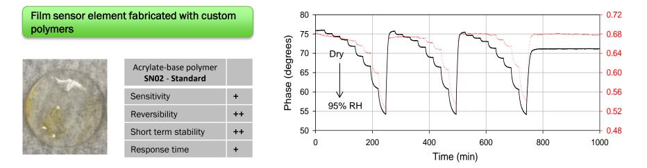
Phase II reformulated sensors based on custom polymers exhibit comparable reversibility, and improved stability and repeatability than those demonstrated in Phase I.
