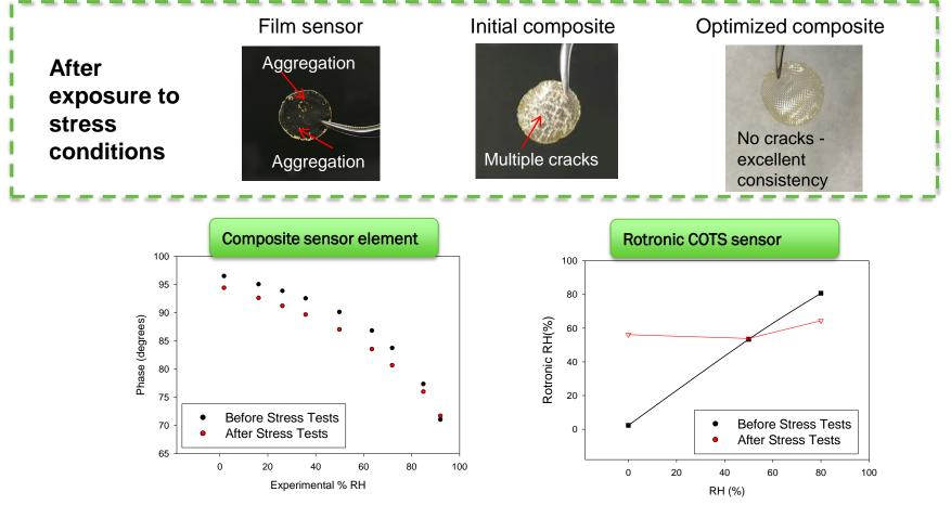
Selected sensor formulations exhibit significantly enhanced resistance to the corrosive environment (salt water) stress test, superior to that of the COTS sensor.
