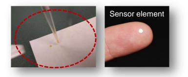
The manufacturing process takes advantage of established biosensor fabrication systems to produce low cost sensors.
