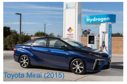
5 kg  $H_2$  + 87.5 kg  $H_2$  storage + 56 kg stack weight = 327 lb total power plant weight 568,000 BTU in the  $H_2$ 1736 BTU/lb thermal ~ 860 BTU/lb electrical (Source: InsideEVs.com)
