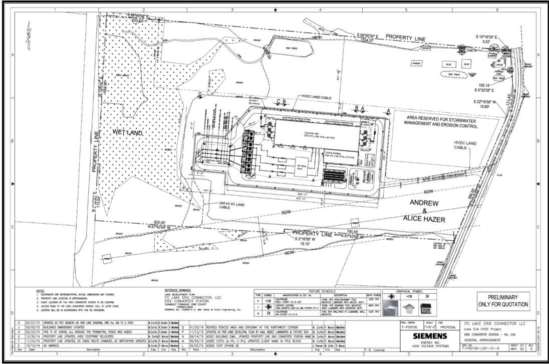
FIGURE 2-6: PRELIMINARY ERIE CONVERTER STATION SITE LOCATION AND LAYOUT
