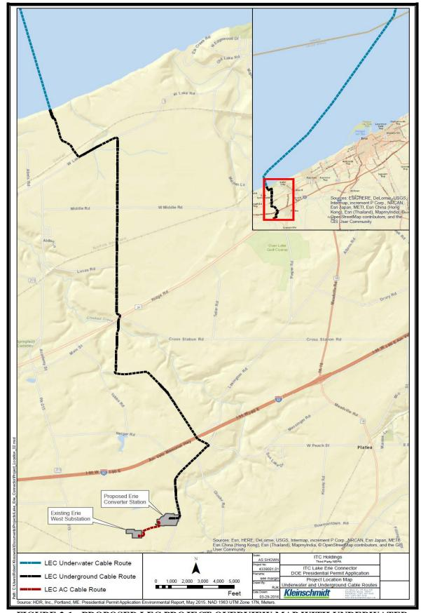
FIGURE 2-1: PROPOSED LEC PROJECT OVERVIEW MAP WITH UNDERWATER AND UNDERGROUND TRANSMISSION CABLE ROUTES
