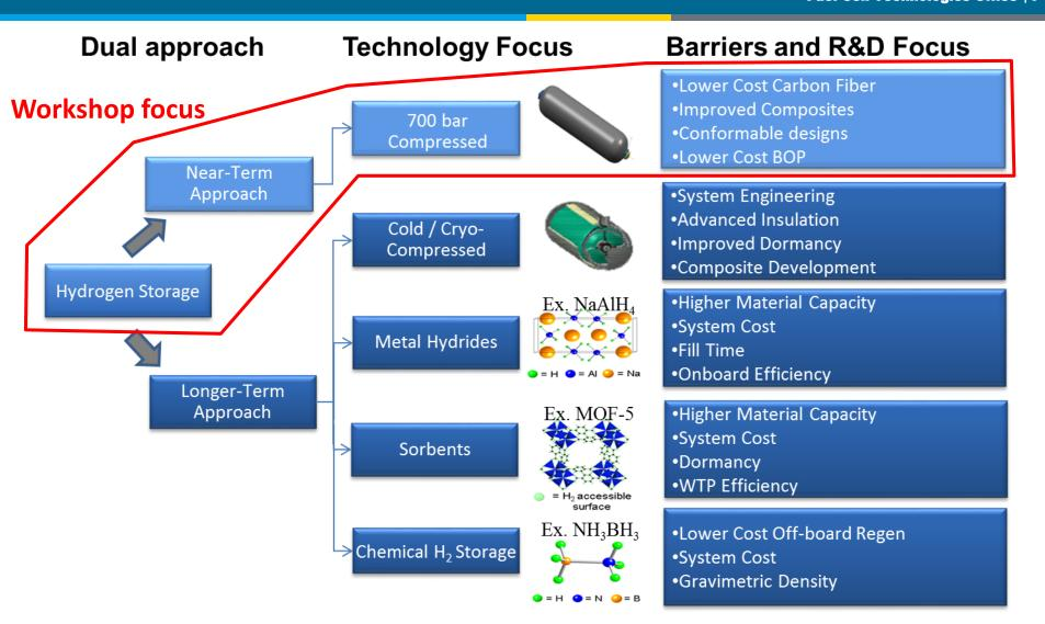
Near-term – address cost and performance of 70 MPa H<sub>2</sub> storage; Long-term – develop advanced technologies with potential to meet all targets
