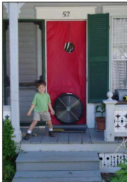
A blower door is required for zone pressure diagnostics
