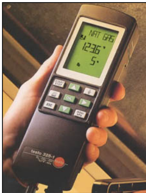
The Testo 325 combustion analyzer measures steady-state efficiency and carbon monoxide emissions
