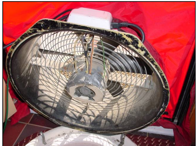
Don't do this! Four small holes in the fan flow sensor ring must be unobstructed and regularly cleared of dust accumulation
