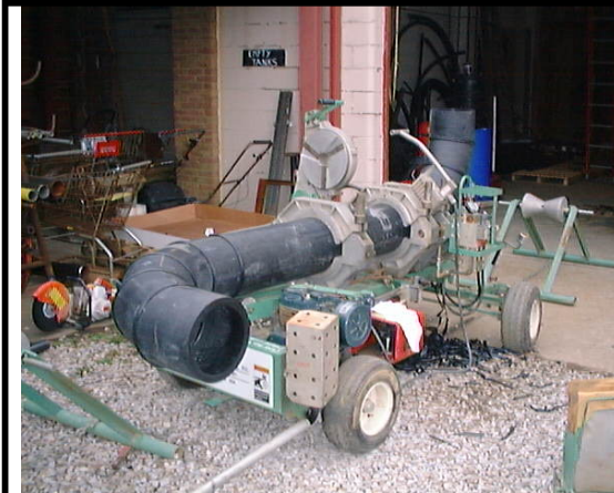
Large Pipe Heat Fusion
