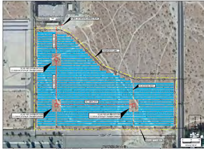
Figure TSPF – 7 ACBCI Allottee Land Ground Mount Solar Project Design – Adjustable Tilt
