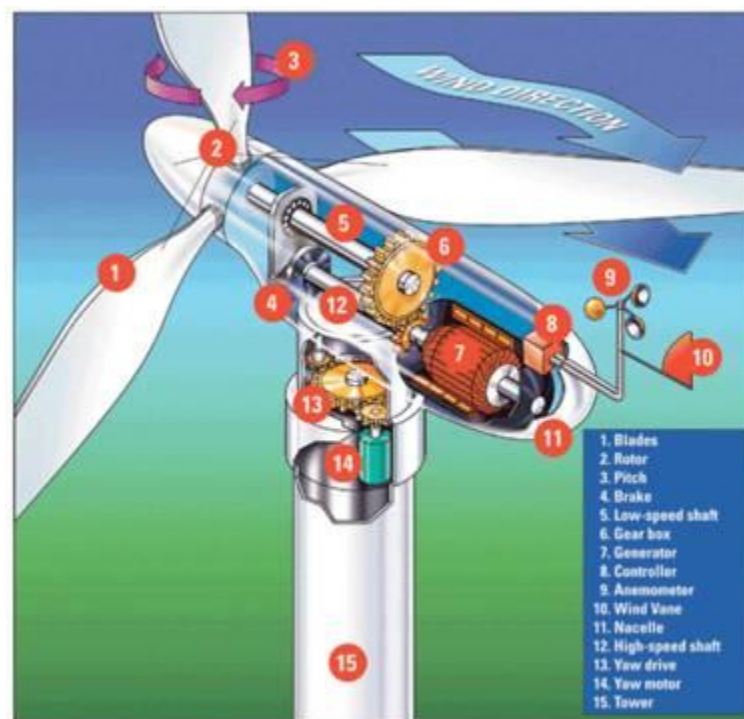
Figure 10 – Wind Turbine Components
