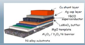
Sub-atmospheric growth process enables reel-to-reel production of long length HTS tapes (BNL Patent)
