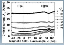
Engineering strong/isotropic pins to achieve record high  $J_c(H)$  and  $T_c$  in YBa<sub>2</sub>Cu<sub>3</sub>O<sub>7</sub> for HTS cables
