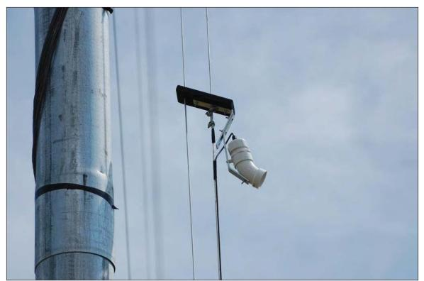
**Photo 5.** High microphone (45m) being raised to pulley bracket.
