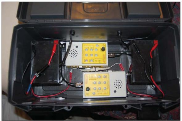
**Photo 2.** ETC design weatherproof housing for 2m and 45m Anabat systems
