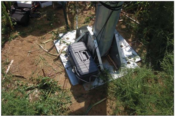
**Photo 4.** Anabat housing at base of MET tower.
