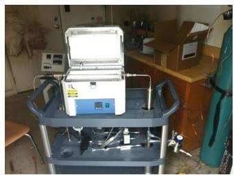
A 10 ml plug flow reactor for testing catalytic tar cracking process
