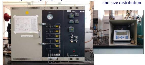
The autoclave engineer's BTRS-JR plug flow reactor unit and four mass flow controllers for testing FT synthesis
