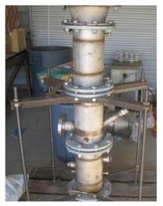
Lab-scale fluidized bed gasifier
