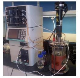
CSRT reactor for preparation of catalysts through co-precipitation
