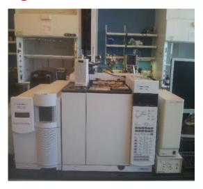
Frontier Micro-Py-GC-MS for testing fast pyrolysis and identifying and quantifying chemicals and biofuels
