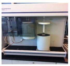
ASAP 2020 BET analyzer for measuring surface area, pore volume
