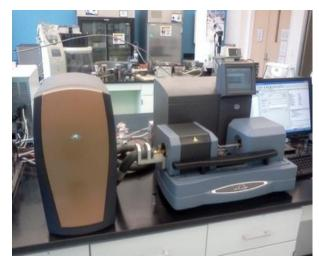
TGA-DSC-MS for measuring thermal degradation characteristics, heat flow and evolving gas profile
