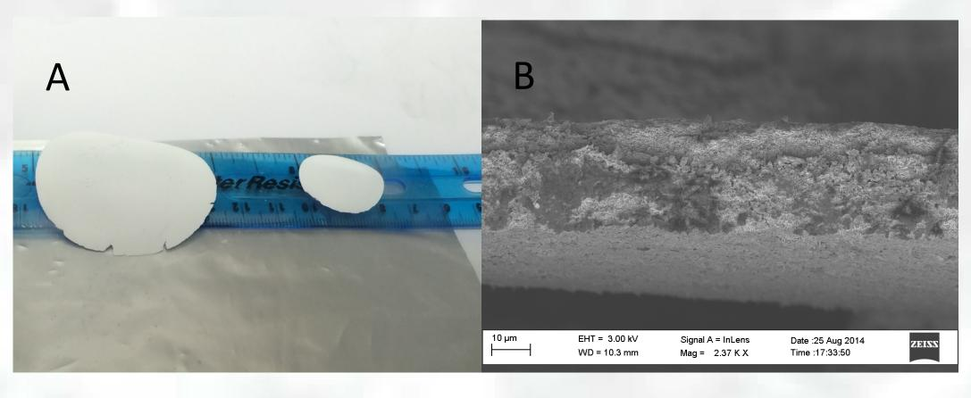
Thin solid electrolyte membranes are crucial for high energy density and excellent cell performance. A slurry coating method has been developed to create freestanding membranes of 2" diameter and 20 µm thickness.
