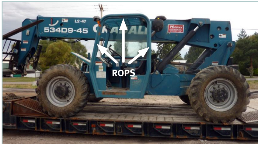
Figure 1-5. Gradall on flatbed after recovery from accident scene shows ROPS intact
