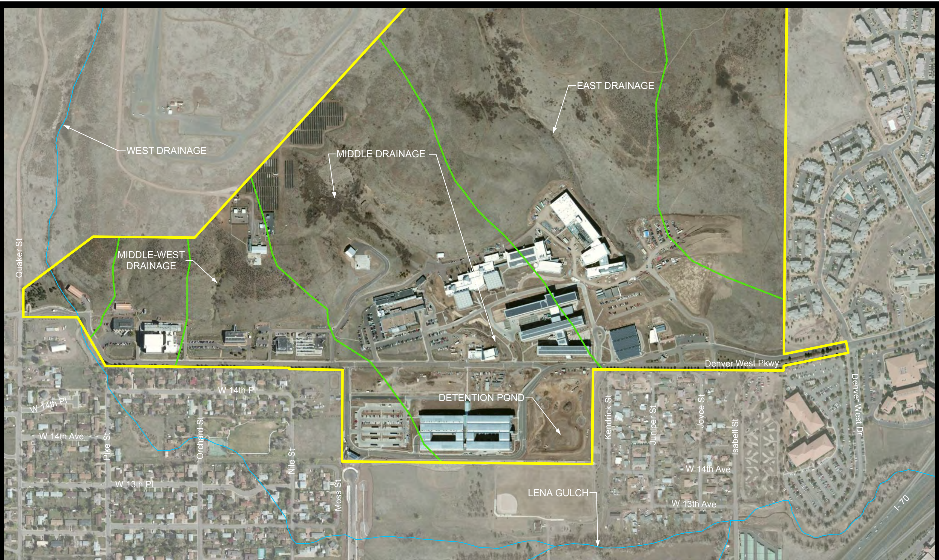
Figure 4-1 - South Table Mountain Upland Swale Drainages
