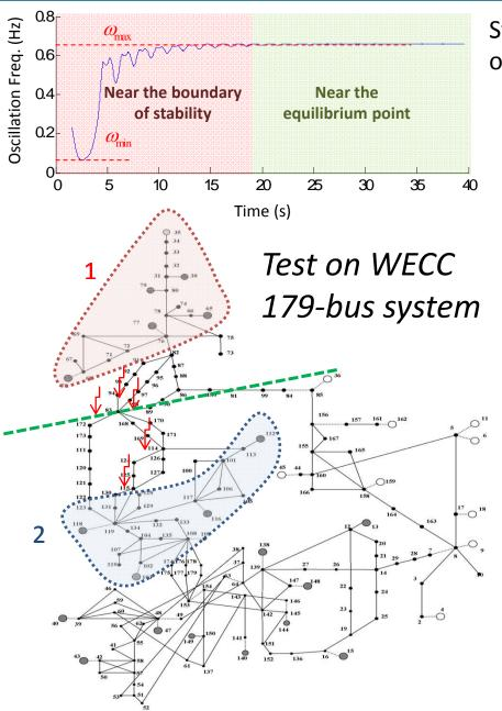
Stability margin index based on fluctuation of the oscillation frequency about a dominant mode
