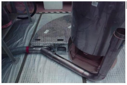
Exhibit 4-1: Ventilation Ductwork for Close Capture System
