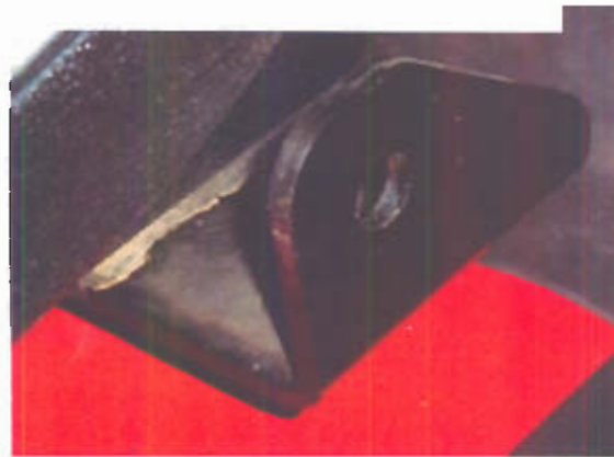
Figure 6. Seat belt attachment bracket (note missing paint in hole and circular scratch marks)
