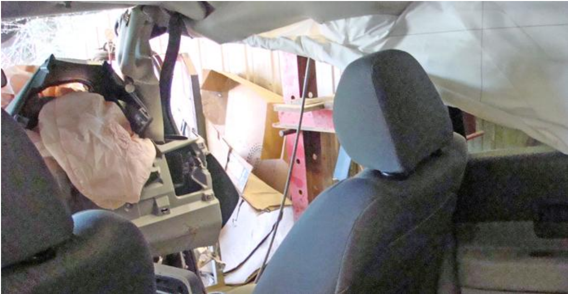
Photo shows that all airbags deployed on impact.
