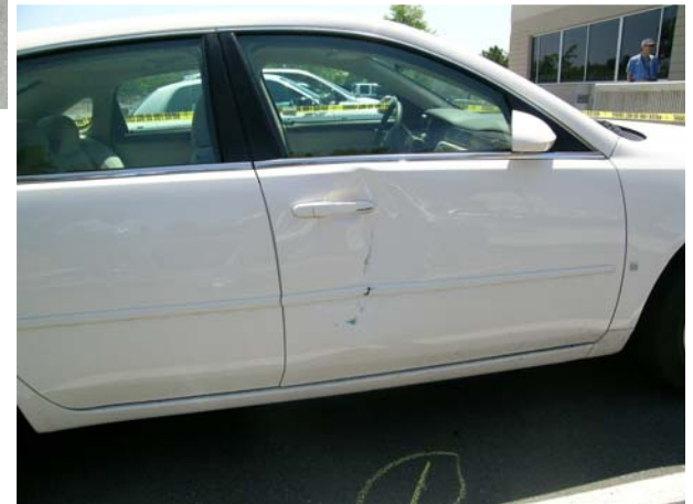
Figure 2-4: Chevrolet Impala (V2) with Damage to Front Passenger Door
