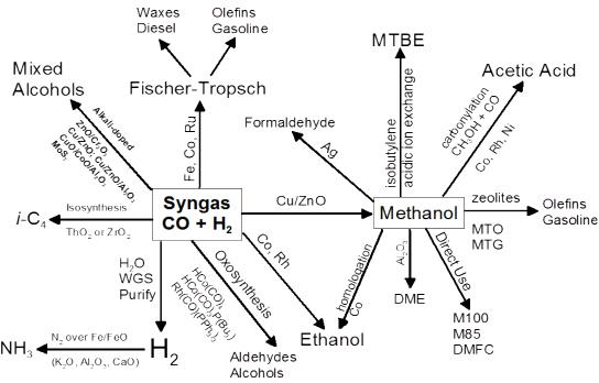
**Figure A6.2:** Known and widely used catalytic pathways to produce chemicals and fuels from a mixture of CO and H<sub>2</sub>.
