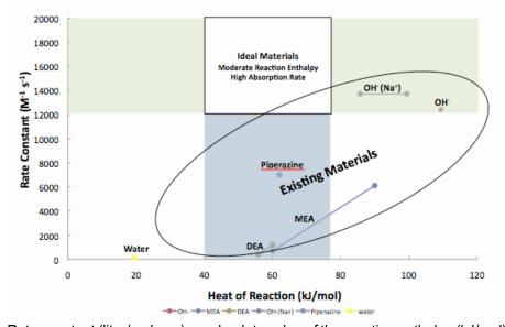
**Figure A8.1:** Rate constant (liter/mol-sec) vs. absolute value of the reaction enthalpy (kJ/mol) for chemical sorbents. Source: APS Report, Figure 3B.1, p. 69.
