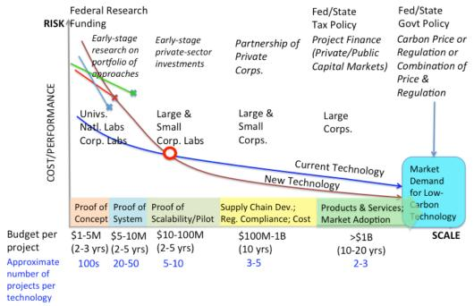
**Figure A3.1** Process of scaling for any technology from research to gigatonne scale expressed as technoeconomic learning curves. New technologies can out-compete current technologies if they are less costly, or have superior performance or offer new services and capabilities. Research based on science and engineering is needed at all stages of this scaling process.
