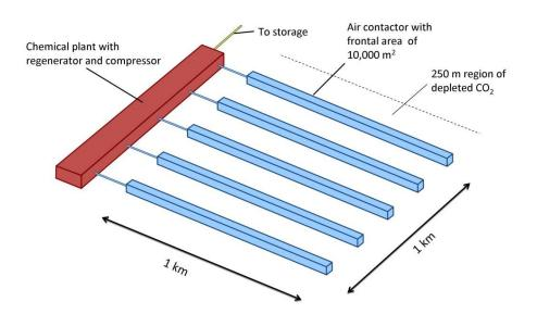
**Figure A9.1:** Schematic representations of a facility for capturing 1 MtCO<sub>2</sub>/yr. The facility could collect 1 MtCO<sub>2</sub>/yr if air passed through at 2 m/s and 50% of the CO<sub>2</sub> were collected. It has five structures, each 10 meters high and 1 km long, and the structures are spaced 250 meters apart. Approximately six of these systems would be required to compensate for the emissions of a 1 GW coal plant. Buildings not to scale. *Source*: APS Report, Figure 1.2B, p. 8.
