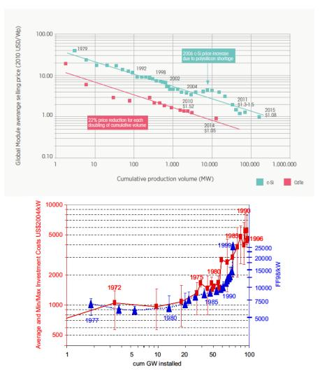
**Figure A3.2 (TOP)** Learning or experience curves of photovoltaic (PV) modules made from crystalline-Si and CdTe (IRENA, 2012). **(BOTTOM)** Cost of nuclear plants (\$/kW) in the US and France (Grubler, 2010)
