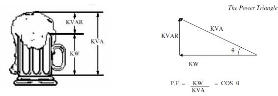
*Figure 2a and 2b*. Model of the beer analogy and the power triangle. Adapted from "Power Factor – The Basics," by PowerStudies, Inc.
