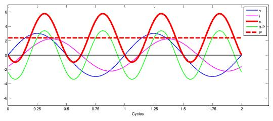
Figure A-3. Power in an AC circuit – general case.
