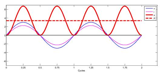
Figure A-1. Power in an AC circuit when voltage and current are in phase.
