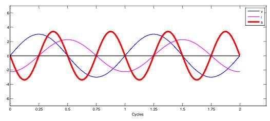
Figure A-2. Power in an AC circuit when current lags voltage by quarter of a cycle.
