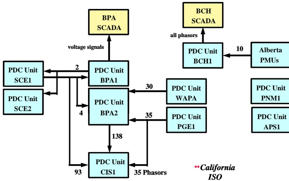
Figure 6. Evolving PDC network in the WECC WAMS
