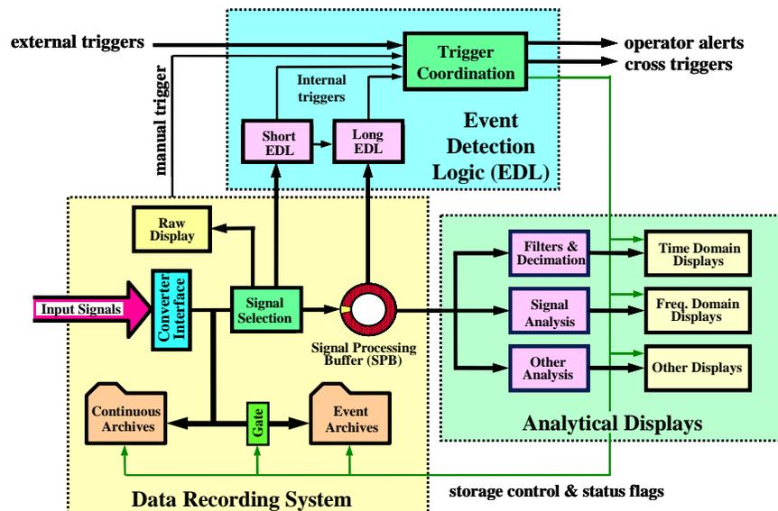
Figure 9. Primary measurement functions of a generic WAMS
