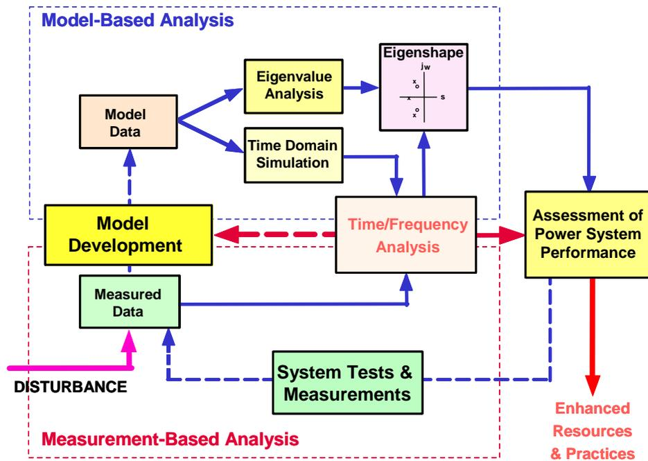
Figure 3. Integrated use of measurement and modeling tools
