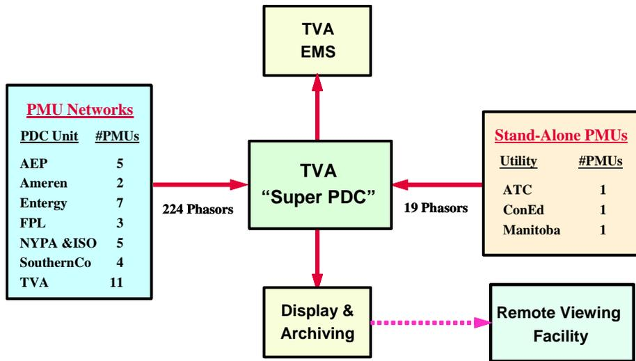
Figure 8. Evolving PDC network in the EI WAMS
