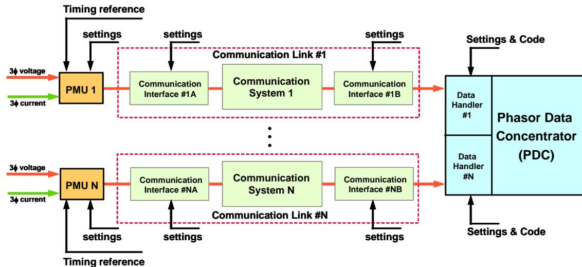
Figure 10. Technology elements for networking PMUs to a PDC
