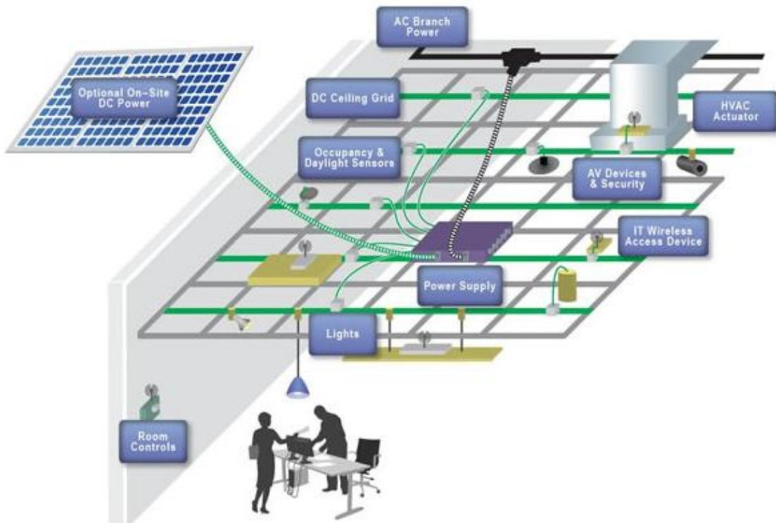
Figure 5. Ceiling DC distribution system architecture block diagram [3].
