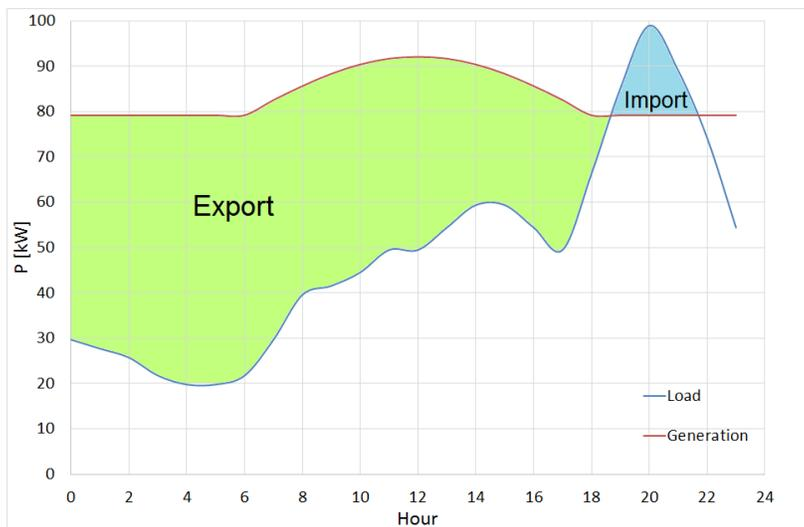
Figure 3: 24-hour Power Supply and Demand Profile of the Microgrid
