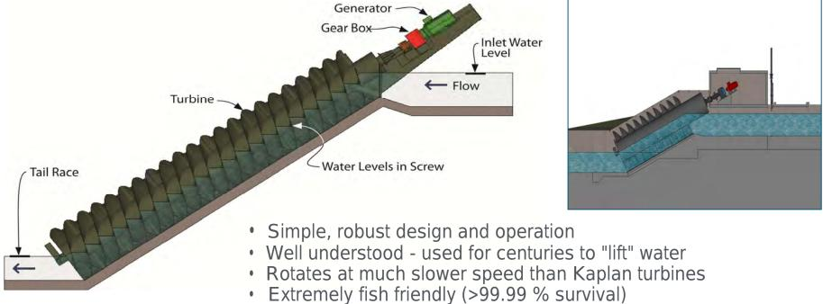
Can tolerate large debris so less trash screening
