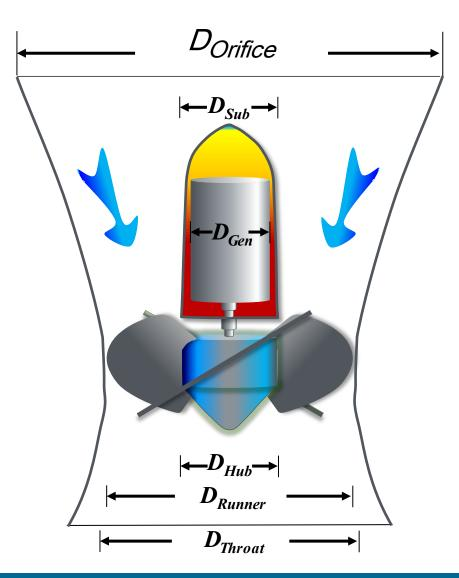
For the off-the-shelf alternator selected, the Venturi parameters are based on the diameter of the alternator and the impeller hub-tip ratio.
