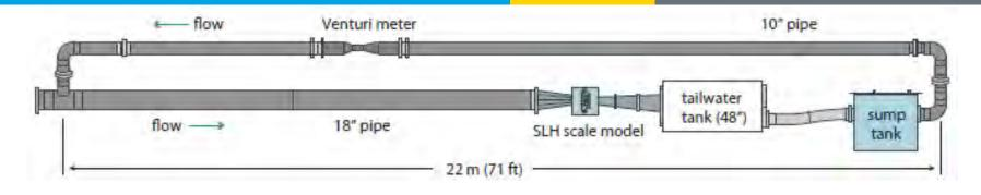
Following recommendations of IEC-60193, PTC 18-2002, and in consultation with Alden, Natel designed, built and commissioned an onsite 1:6.4 scale model hydraulic test facility to confirm CFD-derived loads.
