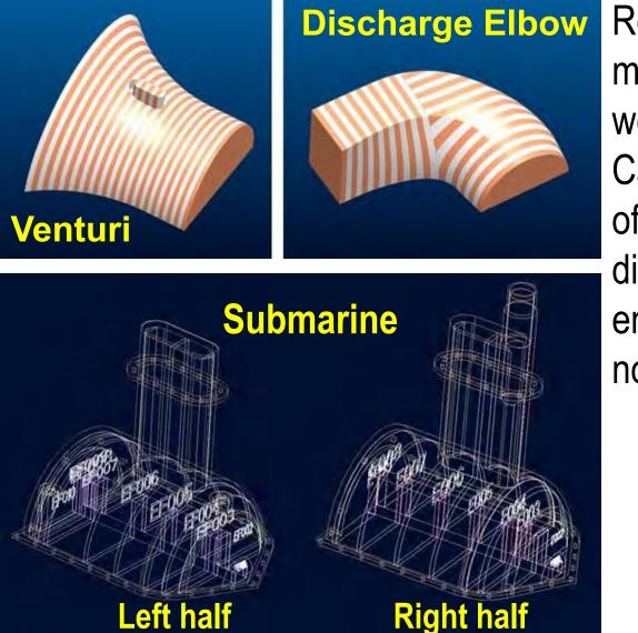
Reusable half-section molds made of Styrofoam and wood are used to fabricate Carbon composite moldings of the Venturi turbine, discharge elbow, submarine enclosure, and impeller nose cone
