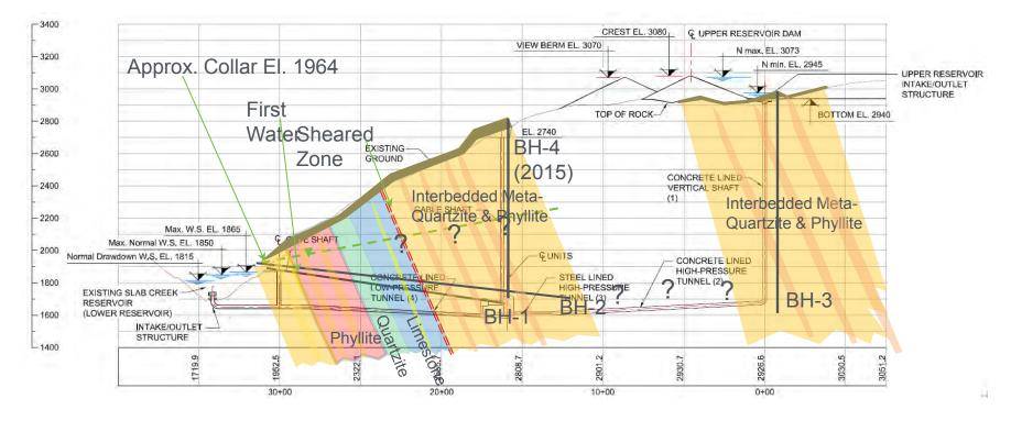
Projected Geologic Profile (based on interpretive geology from Boreholes BH-1 and BH-3)
