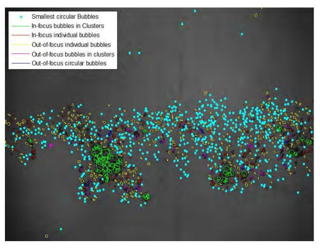
Preliminary calculations based on the current analysis gave a predicted volume flow rate of 0.47 – 0.49 LPM which compares favorably with the 0.5 LPM injected.
