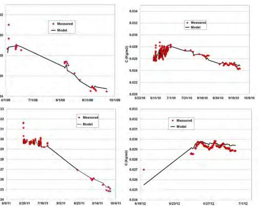
Grand Coulee Tailwater, Measured Vs. Modeled, 2008, 2010, 2011, and 2012
