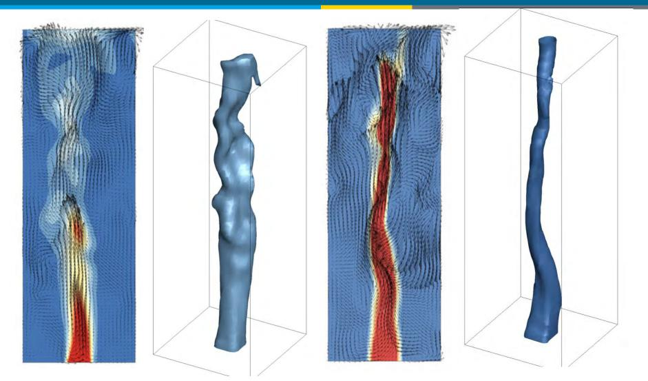
Liquid velocity vectors (left) and iso-surface of gas volume fraction (right) at 2 instants in time
