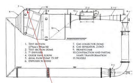
Gas collector dome upstream of test section allows for extended run time with no visible effects on operating conditions
