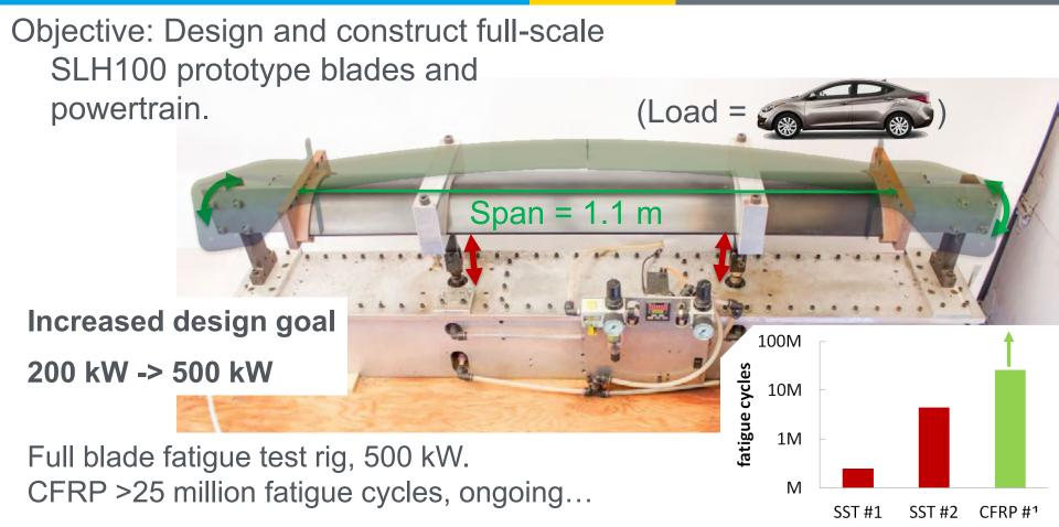
Simulates blade + endplate + clamp + belt attachment system:
