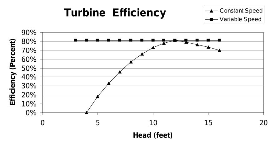
Comparison of Constant Speed and Variable Speed Turbine Efficiencies at variable heads.
