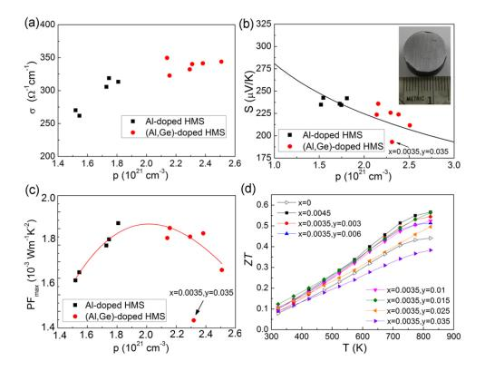
**FIGURE 3.** (a) Electrical conductivity at 800 K, (b) Seebeck coefficient at 800 K, and (c) Peak power factor as a function of the hole concentration at room temperature in  $Mn(Al_xSi_{1,x})_{1,8}$  and  $Mn(Al_{0.0035}Ge_ySi_{0.9965-y})_{1,8}$ , (d) *ZT* values of  $Mn(Al_xSi_{1,x})_{1,8}$  and  $Mn(Al_{0.0035}Ge_ySi_{0.9965-y})_{1,8}$ . Inset of (b) is a photograph of a 15-mm diameter, 8-mm thick disc made by SPS.
