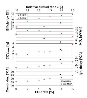
**FIGURE 1.** Trends of Efficiency, NO<sub>x</sub> Emissions, Combustion Stability, Ignition Delay, and Combustion Duration with Increasing Dilution at 2,000 RPM, 6 bar IMEP
