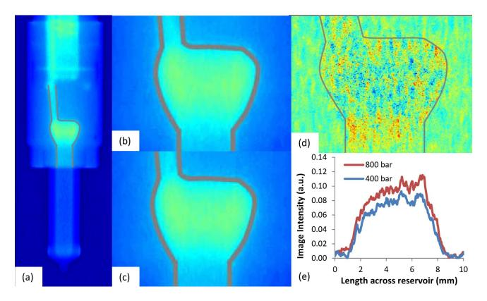
FIGURE 3. Neutron images highlighting the location and density of fuel inside of (a) diesel injectors at (b) 400 bar and (c) 800 bar. (d) Subtracted intensities illustrating a uniform density differences. (e) Graphical representation of the intensities in (b) and (c).
