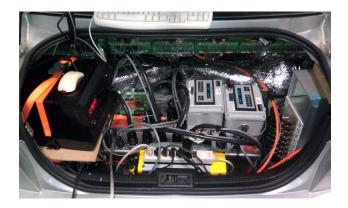
FIGURE 1. Data Acquisition System, TE System Controls, and TE Devices Packaged into the Trunk of the Test Vehicle
