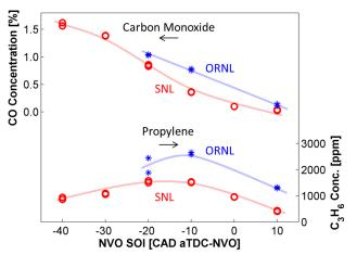
FIGURE 6. Comparison of species concentrations in NVO products measured at ORNL and Sandia under rich NVO conditions.
