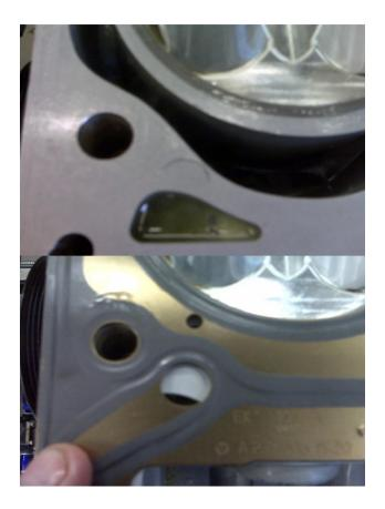
FIGURE 3. Oil Passage Mismatch between ENVERA Engine Block and OEM Cylinder Head Gasket
