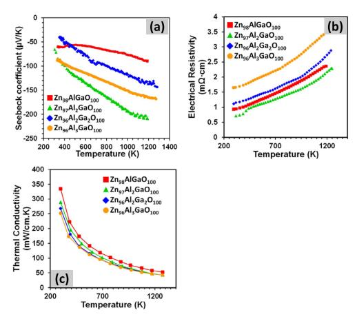
FIGURE 5. Plots showing the variation of (a) Seebeck coefficients, (b) electrical resistivities, and (c) thermal conductivities of dually-doped ZnO nanowire-bulk pellets of various compositions with temperature.
