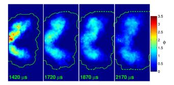
**FIGURE 6.** Average equivalence ratio computed from Rayleigh scatter imaging (calculated for 21% ambient oxygen). The 10% schlieren vapor probability contour is shown by the green line (with dots indicating where the vapor crossed the boundary).
