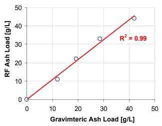
**FIGURE 4.** Comparison of RF and gravimetric measurements of DPF ash load up to 42 g/L. Ash level of 42 g/L corresponds to approximately 240,000 miles of on-road operation.
