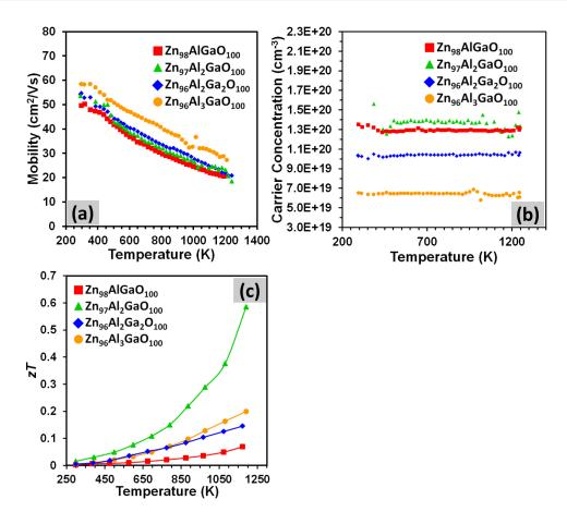
**FIGURE 6.** Plots showing the variation of (a) mobilities, (b) carrier concentrations, and (c) *zT* values of duallydoped ZnO nanowire-bulk pellets of various compositions with temperature.
