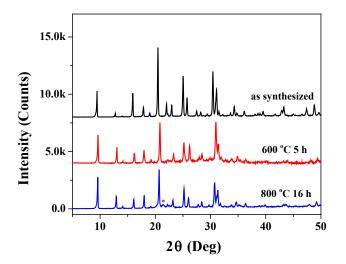
**FIGURE 4.** XRD patterns for the one-pot samples formed using CuO as a Cu source during gel preparation. The as-synthesized sample (dried, prior to structure directing agent removal) and the calcined samples at 600°C for 5 h, and 800°C for 16 h are displayed.
