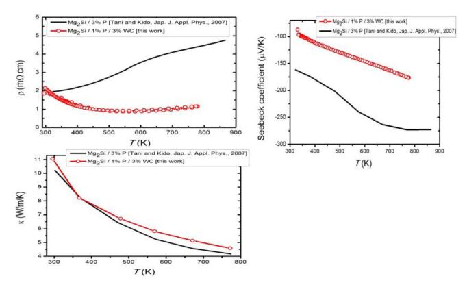
FIGURE 5. Thermoelectric properties of P-doped Mg, Si/WC composite are compared with that of P-doped Mg, Si [3].
