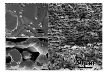
FIGURE 4. Scanning electron micrographs of the layered ZnO materials including the AI nanoprecipitates.
