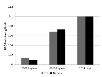
**FIGURE 2.**  $N_2O$  emissions comparison for 2010 and 2007 technology engines relative to the 2014 limit.
