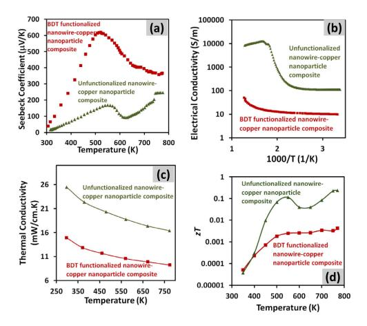
**FIGURE 4.** Plots showing the variation of (a) Seebeck coefficients, (b) electrical conductivities, (c) thermal conductivities, and (d) zT values of both BDT functionalized  $Zn_3P_2$  nanowire-copper nanoparticle composite and unfunctionalized  $Zn_3P_2$  nanowire-copper nanoparticle composite with temperature.
