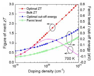
**FIGURE 7.** Calculated ZTs of n-type  $Mg_2Si_{0.4}Sn_{0.6}$  as a function of doping density by the optimal electron energy filtering effect at 700 K. The Fermi level and the optimal cut-off energy level used at each doping density are shown on the right y-axis. The bulk property value is also shown for comparison.
