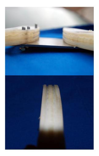
FIGURE 8. Damaged VCR Engine Timing Chain Guides
