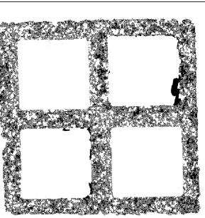
**FIGURE 4.** Processed micro-X-ray CT cross-section of a catalyst filter sample showing the porous substrate in gray and the catalyst in black.
