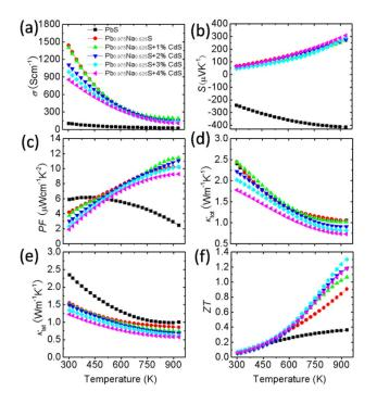
**FIGURE 1.** TE properties as a function of temperature for  $Pb_{0.975}Na_{0.025}S$  with x% CdS: (a) electrical conductivity; (b) thermopower S; (c) power factor; (d) total thermal conductivity; (e) lattice thermal conductivity; (f) *ZT*, the combined uncertainty for all measurements involved in the calculation of *ZT* is less than 15%. Similar results (not shown) were obtained using ZnS, CaS and SrS.
