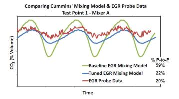
**FIGURE 3.** Comparing transient EGR for Mixer A and a given engine condition as measured by the EGR probe to the EGR Mixing Model results before and after tuning.
