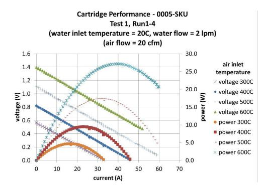
FIGURE 3. Cartridge Voltage vs. Current Curves
