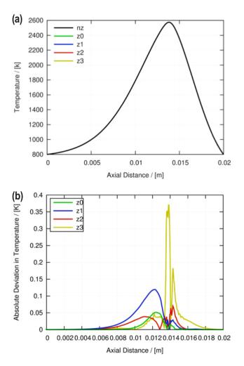
**FIGURE 3.** (a) Temperature versus axial distance for different zoning strategies, and (b) difference in axial temperature for different zoning strategies relative to the every cell simulation.
