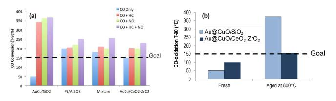
FIGURE 6. Summary of Tank light-off temperatures as they are affected by (a) exhaust constituents and (b) hydrothermal aging.
