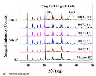
FIGURE 3. XRD patterns of the SAPO-34/CuO physical mixture and the SSIE samples. Calcination conditions are listed adjacent to the XRD patterns.
