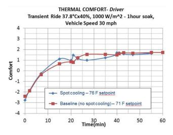
FIGURE 3. Equivalent thermal comfort comparison between TE-equipped vehicle and the baseline.
