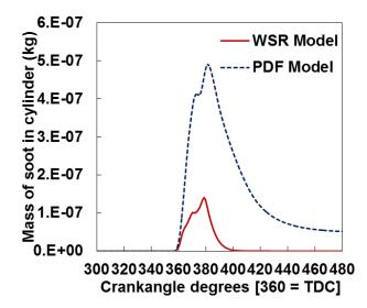
**FIGURE 5.** Computed (WSR versus PDF models) in-cylinder soot mass as a function of crank angle for a full-load, high exhaust gas recirculation operating condition.
