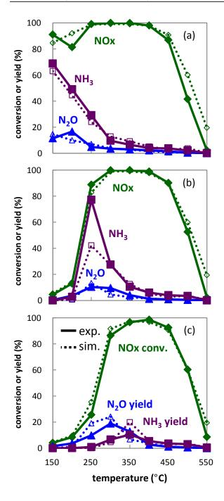
**FIGURE 2.** Flow reactor measurements (solid lines and filled symbols) and ICT Prague model predictions (dashed lines and open symbols) of cycle averaged NOx conversion (green diamonds), NH<sub>3</sub> yield (purple squares), and N<sub>2</sub>O yield (blue triangles) as a function of temperature and reductant composition: (a) H<sub>2</sub>, (b) CO, and (c) C<sub>3</sub>H<sub>6</sub>. Operating conditions: same as in Figure 1.
