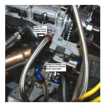
FIGURE 5. Added Oil Supply Line from Engine Block to Cylinder Head
