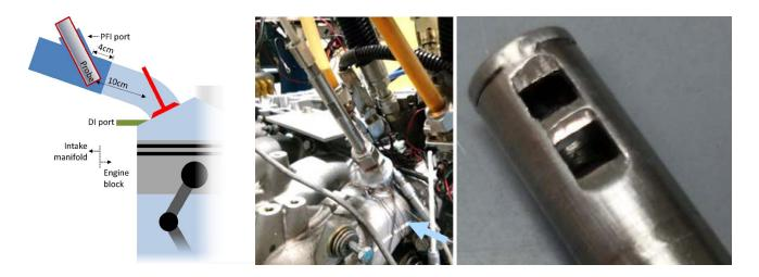
FIGURE 4. Schematic (left) of the single-cylinder engine and picture (center) of the EGR probe installed in the intake runner. The EGR probe (right) was modified to incorporate chamfers along the flow-orientation axis as recommended by computational fluid dynamics analysis.
