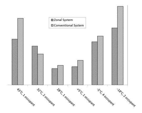
FIGURE 6. Relative Energy Consumption of HVAC System Measured during Wind Tunnel Evaluations
