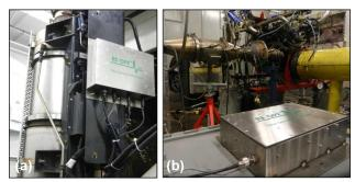
**FIGURE 2.** RF sensors prototype and control unit installed next to DPF on the exhaust stack of a heavy-duty truck for fleet testing (a) and installed on a light-duty General Motors engine at Oak Ridge National Laboratory (b).
