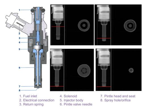
FIGURE 4. Comparison of cutaway view of a GDI-based injector, with one based on a CT scan build from neutron images.
