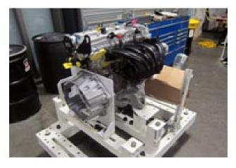
FIGURE 3. Engine Installation on a Test Cell Cart at Clemson University
