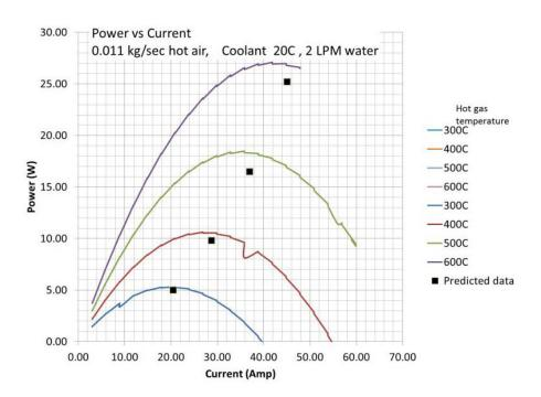
FIGURE 2. Cartridge Power vs. Current Curves
