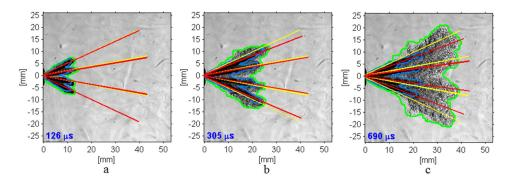
**FIGURE 3.** Time sequence of injection. Ambient: 900 K, 3 kg/m<sup>3</sup>, 0% O<sub>2</sub>. Injection: iso-octane, 200 bar, 0.87 ms injection duration. Vapor and liquid envelopes are shown in green and blue, respectively. Drill angles and plume vectors are shown in yellow and red, respectively
