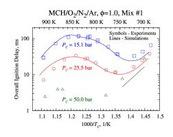
Comparison of the methylcyclohexane model with experimental ignition data from a rapid compression machine, for a stoichiometric mixture, over a range of temperatures, and at pressures of 15, 25 and 50 bar. (Pitz, LLNL)
