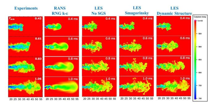
FIGURE 3. Fuel vapor temperature contours using RANS RNG k- $\varepsilon$  and different LES models at a minimum mesh resolution of 0.0625 mm compared against experimental data from Sandia National Laboratories [2] using n-heptane as a surrogate for diesel fuel.
