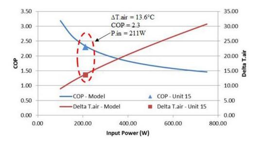
FIGURE 3. Calorimeter Performance and Efficiency of TE Device in Cooling Mode
