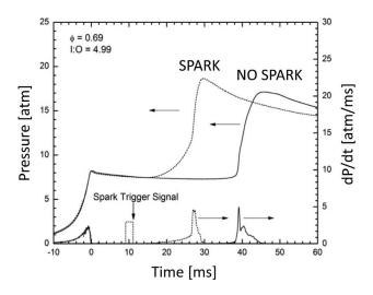
**FIGURE 6.** Pressure traces from the RCF showing the effect of spark on ignition delay with iso-octane:  $O_2$ :  $N_2$  mixture at 7.9 atm. Testing over a wide range of conditions was used to establish limiting conditions for SACI.
