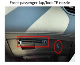
FIGURE 1. Nozzles for TE HVAC components in the Buick LaCrosse demonstration vehicle.
