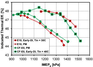
**FIGURE 3.** Comparison of gross indicated TE for Early-DI PFS and premixed (PM) fueling as a function of IMEP<sub>g</sub> at P<sub>in</sub> = 2.4 bar and RI ≈5 MW/m<sup>2</sup>, 1,200 rpm. For premixed fueling,  $T_{in} = 60^{\circ}$ C, and for Early-DI PFS,  $T_{in} = 30$  or 40°C as noted in the legend.
