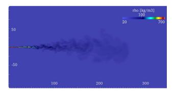
**FIGURE 3.** Instantaneous density field along the center plane of the jet at 0.27 ms. The spatial scale is non-dimensionalized using the jet diameter of 0.09 mm.
