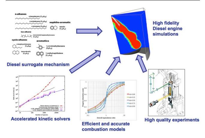
FIGURE 1. Schematic of the approach to advanced engine combustion simulation combining detailed chemical kinetics, advanced solvers, advanced combustion models, and high quality experiments.
