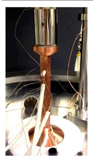
FIGURE 5. High-temperature one-dimensional reference bar thermal interface test rig.
