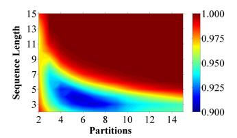
**FIGURE 1.** Variation of Modified Shannon Entropy with Number of Partitions and Sequence Length for 2,000 rpm, 3.8 Bar Brake Mean Effective Pressure Operation with 17% EGR
