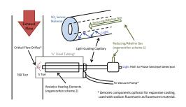
The probe concept can exploit expansive cooling from atmospheric to near-vacuum pressure, and a light-guiding capillary allows the sol gel containing a material, copper zeolite, sensitive to SO<sub>3</sub> and to be interrogated with laser induced luminescence and regenerated with an alkaline gas. (Partridge, ORNL)
