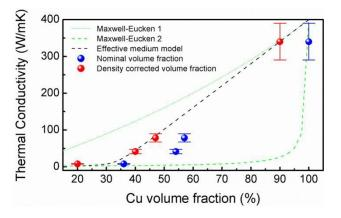
**FIGURE 4.** Thermal conductivity as a function of Cu volume fraction for hot-pressed Cu-ZrW<sub>2</sub>O<sub>8</sub> composites. After correcting for porosity based on independent density measurements, the experimental data show excellent agreement with the effective medium model (dashed black line). The trends predicted by the Maxwell-Eucken model (dotted and dashed green lines for the upper and lower limit, respectively) are also shown for comparison.
