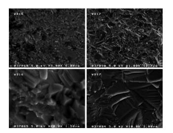
**FIGURE 2.** SEM images of the methanol-etched fracture faces of 1.0% Yb doped  $Mg_2Si$  (left) and 1.0% Bi doped  $Mg_2Si$  (right). The two left images show the microstructure of a sample sintered at 750°C using 5k (top left) and 20k (bottom left) magnification. The images on the right were taken on a sample sintered at 700°C but prepared by a short ball mill approach. The top right one was taken at a magnification of 1.8k, the bottom right one at 10k.
