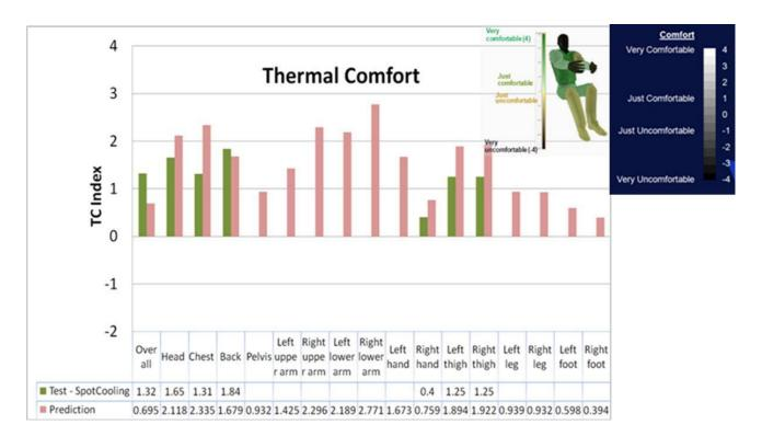
FIGURE 2. Thermal comfort CAE tool validation results for one of the spot cooling test conditions.
