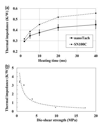
**FIGURE 3.** Plots of transient thermal impedance vs. (a) heating pulse width measured on power packages having chips bonded by nanosilver sintering (nanoTach) and lead-free soldering, and (b) die-shear strength with nanosilver-bonded joints showing that a minimum of 10 MPa bonding strength is necessary for high thermal performance of the sintered joint.
