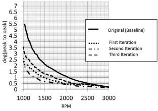
FIGURE 6. Reduction in 2<sup>nd</sup> Order Torsional Vibration at Full Load
