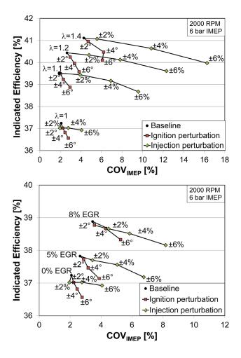
FIGURE 2. Effect of Injection and Ignition Perturbation on Combustion Stability and Efficiency in Lean (top) and EGR-Dilute (bottom) Operation
