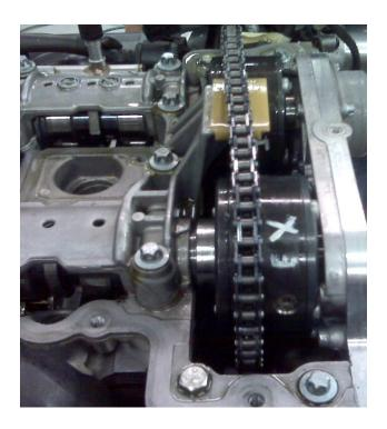
FIGURE 2. Failed Exhaust Cam Phaser Mechanism
