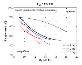
**FIGURE 6.** Comparison between the measured and computed minimum ignition temperatures as O<sub>2</sub> concentration and pilot mass are varied.
