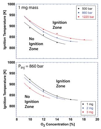
**FIGURE 3.** Impact of injection pressure and pilot injection mass on the minimum charge gas temperature needed to obtain a robust ignition event, for various charge gas  $O_2$  concentrations.
