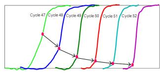
FIGURE 6. Experimental Hybrid Combustion Mass Fraction Burned Curves during the SI-HCCI Mode Transition
