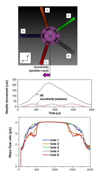
**FIGURE 1.** Three-dimensional transient simulation of a multi-hole injector with specified needle lift and wobble profile. The differences in mass flow rates between different orifices are clearly observed, especially during the needle transients.
