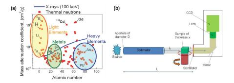
(a) Mass attenuation coefficients of a range of elements as a function of atomic number. Comparison given between neutron (squares) and X-rays (line). (b) Schematic of a neutron imaging facility at ORNL. (Toops, ORNL)
