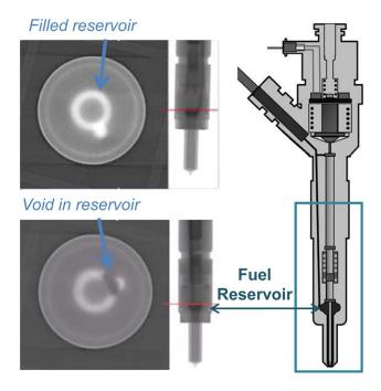
**FIGURE 2.** Cutaway diagram of a commercial diesel fuel injector and the corresponding image obtained with neutron radiography. Areas of highest contrast are associated with hydrocarbons inside metal fuel injector. (left) Virtual cross-section of two fuel injectors, one with the reservoir filled (top) and another with a void (bottom).
