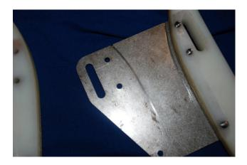
FIGURE 9. Chain Rub and Damage to Guide Support Plate
