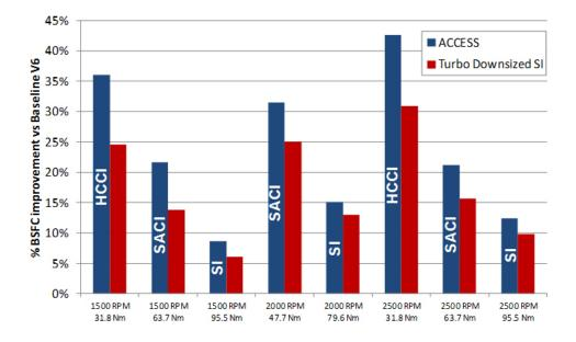
FIGURE 2. Fuel Efficiency Improvement Observed on the ACCESS Prototype II Engine at Frequently Visited Driving Cycle Operation Points
