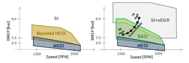
FIGURE 1. Combustion Modes and Associated Operation Ranges
