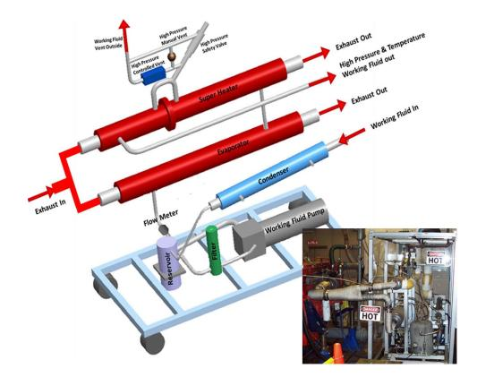
FIGURE 2. Expander Test Setup
