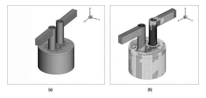
FIGURE 3. Starting grid (a) and final refined grid (b) when simulating a 2-valve engine using hp-adaptive PCS FEM system.
