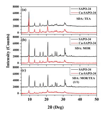
**FIGURE 2.** XRD patterns for SAPO-34, and Cu-SAPO-34 samples prepared by IE. SAPO-34 samples were formed using (a) TEA, (b) MOR and (c) mixed (MOR/TEA = 1/1) structure directing agents.
