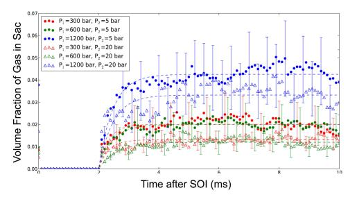
**FIGURE 4.** Plot showing the volume fraction of gas bubbles in the injector sac versus time after start of injection. The volume of gas quickly rises after the end of injection, then stabilizes. The gas fraction is shown for several injection and ambient pressures.
