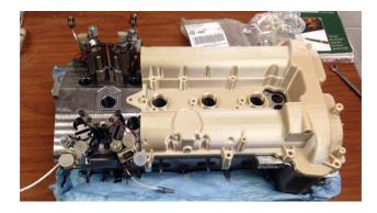
FIGURE 6. Cylinder head and custom valve cover for flexible ORNL multicylinder engine experiment that will be completed during FY 2014.
