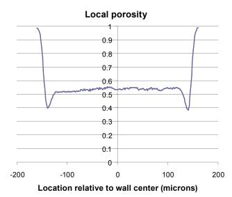
FIGURE 5. Variation of local porosity across the thickness of a single cordierite filter wall.
