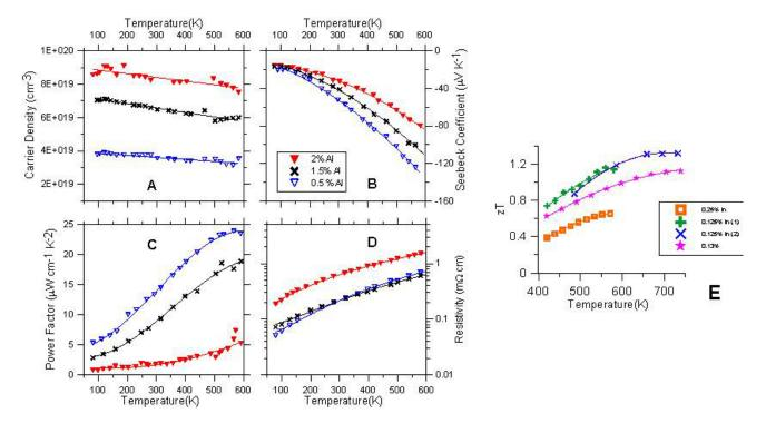
**FIGURE 2.** TE properties of  $Pb_{1,x}Al_xSe$  with 0.5% < x < 2%: carrier density (A), thermopower S; (B), power factor (C) and electrical resistivity (D) vs. temperature (77-600 K). Similar data are obtained on  $Pb_{1,x}In_xSe$  (E) the *ZT* for  $Pb_{1,x}In_xSe$  reaches >1.2 and has a broad maximum at T≥600 K.
