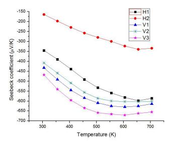
FIGURE 3. Seebeck of Mg,Si by VPS and Hot Press
