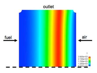
**FIGURE 2.** Temperature contours for two-dimensional laminar opposed laminar non-premixed reactor used for testing the multi-zone combustion model.
