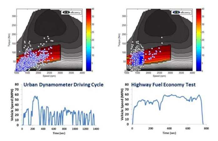
FIGURE 2. RCCI Coverage of Various Drive Cycles with Engine Speed and Load Points Overlain
