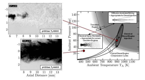
**FIGURE 1.** Regime diagram for n-dodecane injected at a temperature of 363 K into nitrogen suggests the presence of dense supercritical jets under diesel engine conditions without drop formation. High-speed imaging of both a dense jet and spray illustrates the significant transitional change that occurs at high supercritical pressures (images courtesy of L.M. Pickett, Sandia National Laboratories, Combustion Research Facility).
