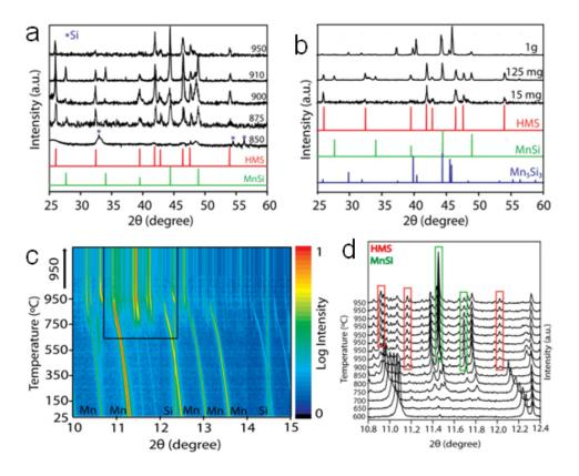
**FIGURE 2.** (a) Powder X-ray diffraction patterns of NW arrays converted at 850, 875, 900, 910, and 950°C, (b) Powder X-ray diffraction patterns of converted NW arrays made with 15, 125, and 1,000 mg of Mn precursor, (c) In situ high-resolution powder X-ray diffraction contour plots showing the silicidation process of Si NW, (d) selected high-resolution powder X-ray diffraction patterns in the region highlighted in (c) showing the emergence of MnSi and HMS during the heating process.
