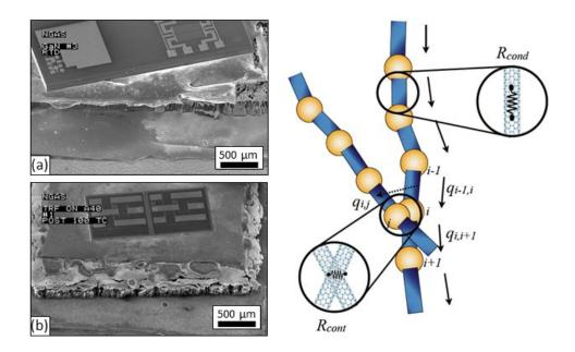
**FIGURE 1.** (left) Scanning electron micrographs of electronic test devices, including (a) a GaN-based device and (b) a thin-film resistor device. These devices are attached to substrates using reactive metal-bonded CNT TIMs. (right) Representative nodal network for CNT coarse-grained model.
