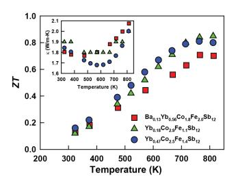
**FIGURE 3.** Temperature dependent *ZT* for double- or mono-filled Fe substituted skutterudites. Inset figure shows temperature dependent thermal conductivity,  $\kappa$ , for the three skutterudite specimens.
