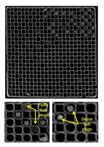
FIGURE 5. One section of a full-size SiC diesel PF containing ash plugs with varying densities, "fluffy" and "dense".
