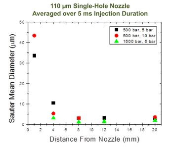
**FIGURE 5.** Sauter mean diameter of fuel parcels in the spray versus distance from the nozzle for two different ambient and injection pressures. These measurements were performed using X-ray small angle scattering, a new diagnostic for measuring particle size in the near-nozzle region. The results were obtained from a 110-µm single-hole nozzle.
