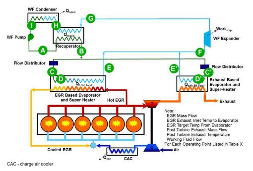
FIGURE 6. Waste Heat Recovery System - Parallel Architecture
