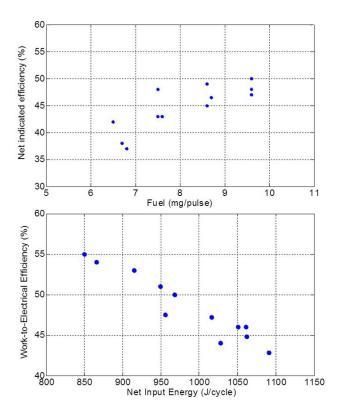
FIGURE 6. Efficiency Trends From Combustion Experiments
