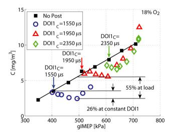
**FIGURE 2.** Measured engine-out soot expressed as carbon (C) concentration for a duration sweep of single injections (filled black squares) and three post-injection duration sweeps (open symbols) added to three different single-injection conditions at 18% intake oxygen fraction.
