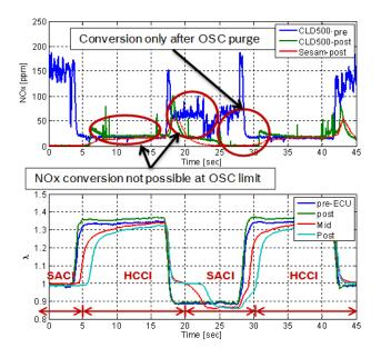
FIGURE 4. Aftertreatment Performance during HCCI–SACI Mode Switches on the ACCESS Prototype II Hardware
