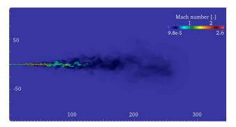
**FIGURE 4.** Instantaneous Mach number field along the center plane of the jet at 0.27 ms. The spatial scale is non-dimensionalized using the jet diameter of 0.09 mm.
