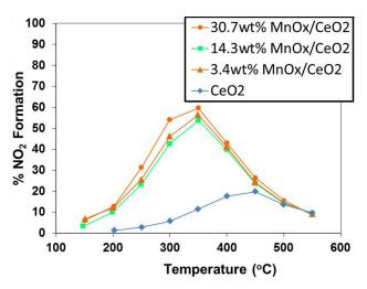
**FIGURE 2.** Effect of Mn loading on the activity of  $MnO_x/CeO_2$  catalysts prepared by incipient wetness impregnation after aging. Aging was performed in 10% steam in air at 700°C for one hour. Reaction conditions: 50 mg catalyst, 156 sccm total flowrate, gas composition: 200 ppm NO, 10% O<sub>2</sub>, 10% steam, balance N<sub>2</sub>.
