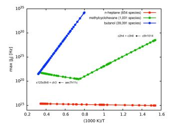
**FIGURE 1.** The new tool identifies the fastest reaction timescales using the Jacobian information from the adaptive preconditioner method during a simulation to provide an extra level of error-detection in mechanism development.
