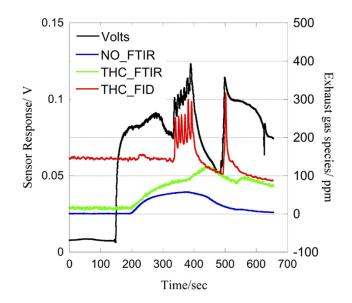
FIGURE 4. Sensor response at 0.0  $\mu$ A bias to engine exhaust when operated in Premixed Charge Compression Ignition mode. The THC measured by an FID is plotted along with the THC and NO measured by a downstream FTIR.
