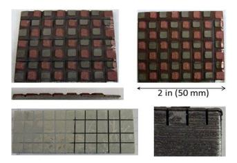
FIGURE 5. TEG Prototype Fabricated Using Thermal Spray
