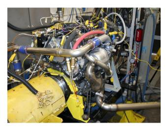
FIGURE 3. LPL EGR Turbocharged Engine Test Cell Installation
