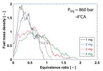
**FIGURE 5.** Fuel mass distributions measured for the conditions corresponding to the apparent heat release traces shown in Figure 2.
