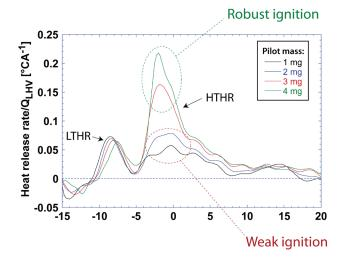
**FIGURE 2.** Normalized apparent heat release rate associated with the pilot injection alone, for various pilot injection quantities at an injection pressure of 860 bar. The presence of a pronounced high-temperature heat release peak corresponds to a "robust" ignition event.
