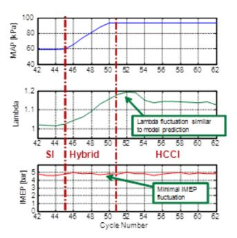
**FIGURE 5.** IMEP and Air/Fuel Ratio during the Combustion Mode Transition Responses
