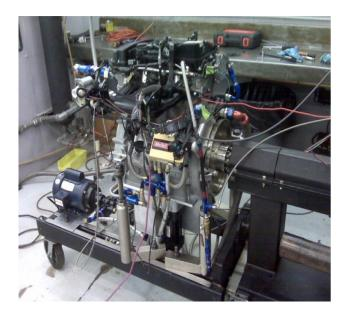
FIGURE 1. VCR Engine at Automotive Specialists Dynamometer Stand
