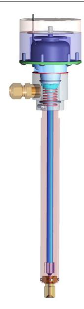
FIGURE 1. Schematic of Sandia dump valve assembly.
