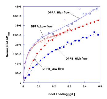
FIGURE 3. Pressure drop build-up during filtration for two different filters at two different flow rates.
