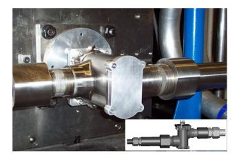
FIGURE 1. Single-Stage Roots Expander
