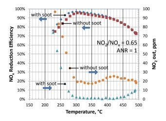
**FIGURE 2.** NO<sub>x</sub> reduction performance and post-filter NO<sub>2</sub> concentration with simulated exhaust versus temperature for NO<sub>2</sub>/NO<sub>x</sub> = 0.65, 150 g/L SCR catalyst loading, with and without 4 g/L initial soot loading, 500 ppm NO<sub>2</sub>, ANR = 1, 35,000 GHSV.
