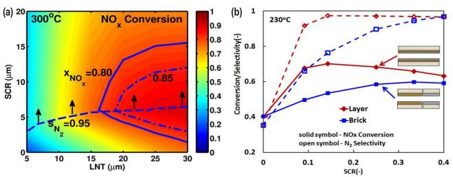
Impact of catalyst loading on NOx conversion in dual-layer catalyst (left). Comparison of performance of dual-layer and dual-brick configuration (right)
