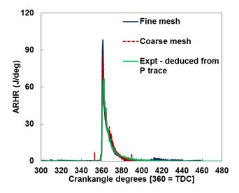
**FIGURE 3.** Heat-release profiles for a baseline diesel case at part load. Mesh sensitivity of the CFD heat-release prediction is also shown in the heat-release profiles.
