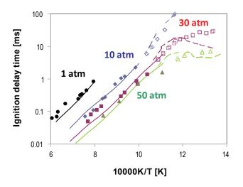
FIGURE 1. A comparison of ignition behavior from the chemical kinetic model (curves) and the experiments (symbols) for n-butyl benzene. The solid curves and closed symbols are results from the shock tube and the open symbols and the dashed curves are from the RCM.
