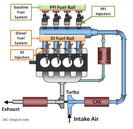
FIGURE 1. ORNL Multi-Cylinder RCCI Engine
