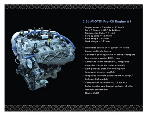
FIGURE 1. Multi-Cylinder Engine Build
