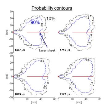
**FIGURE 4.** Vapor probability contours (10% and 90%) at 700 K, 6 kg/m<sup>3</sup> conditions. Contours are derived from schlieren vapor envelopes. Dots show where the vapor crossed the field of view boundary. The red asterisk indicates the injector tip, and the red line is the laser sheet location.
