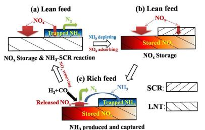
FIGURE 4. Schematic of the working principle of the dual component layered catalyst.
