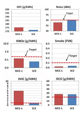
**FIGURE 1.** GDCI Combustion Results at 2,000 RPM-11 Bar IMEP for Multi-Cylinder Development Engine (red) And Single-Cylinder Concept Engine (blue)
