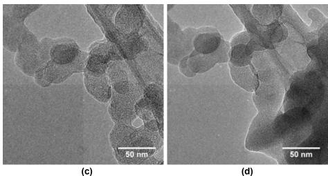
**FIGURE 1.** (a) Particle number distributions, (b) Observation of nanoparticles  $\leq 20$  nm, (c) and (d) Observation of high concentration of volatile organics from the GDI engine.
