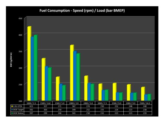
FIGURE 2. Engine Fuel Consumption
