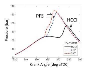
**FIGURE 4.** CFD simulations comparing in-cylinder pressure for HCCI (solid curve) and PFS mode (dashed) at 2 bar intake pressure. Inflected PFS pressure curves indicate two-stage burning caused by LTHR in the richer parts of the charge and the resulting alteration in the temperature-equivalence ratio distribution. Dashed labels denote the crank angle at SOI.
