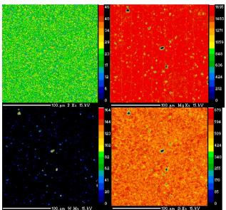
**FIGURE 4.** Electron probe microanalysis X-ray maps showing P, Mg, Si and W distribution in P-doped Mg,Si/WC sample (from left to right).
