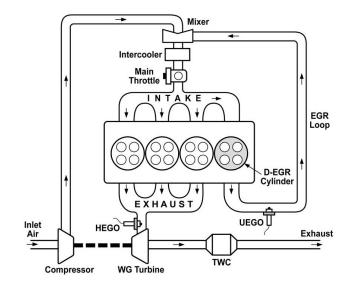
FIGURE 5. D-EGR System Applied to Turbocharged Engine
