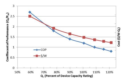
FIGURE 5. Correlation between Cost and Thermal Capacity of TE Devices for Heating and Cooling
