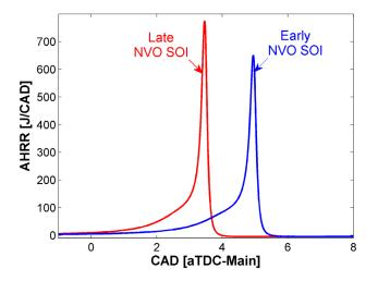
FIGURE 5. Chemical kinetics simulation of apparent heat release rate for main combustion. The two curves represent an early and a late NVO SOI case.
