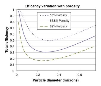
FIGURE 4. Expected variation of filtration efficiency with porosity in a typical cordierite filter.
