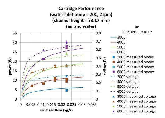
FIGURE 4. Cartridge Voltage and Power vs. Air Mass Flow
