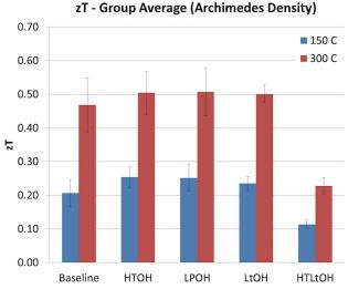
**FIGURE 3**. Measured ZT values for n-type Mg-Si elements from a sintering process study. Results were consistent for the high-temperature (HTOH), low-pressure (LPOH), and low-time (LtOH) cases, while the high-
