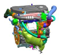
Low-Pressure Loop EGR System Packaged in GM Mid-Sized Vehicle (Keating, General Motors)
