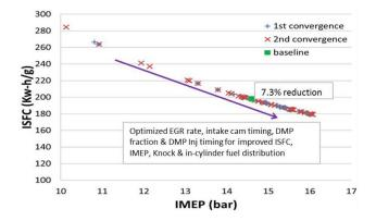
FIGURE 4. Genetic Algorithm Simulation Results—Fuel Consumption
