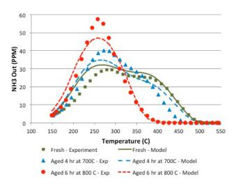
$\mathbf{FIGURE~1.~NH}_{3}$  release from Cu-CHA catalyst during TPD at various aging states.
