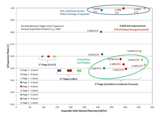
FIGURE 4. Architecture 4 – Three-Stage Expander System BSFC Improvement
