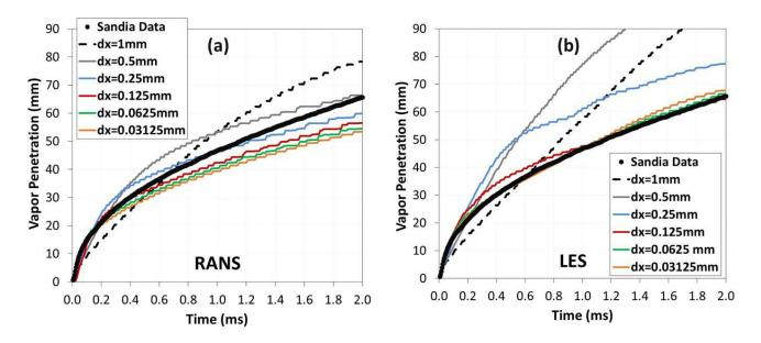
FIGURE 2. Fuel vapor penetration using RANS RNG k-ε and LES dynamic structure models at different minimum mesh resolutions compared against experimental data from Sandia National Laboratories [2] using n-dodecane as a surrogate for diesel fuel.
