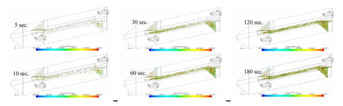
FIGURE 5. The predicted 3-D distributions of particulates during filtration at different filtration times.
