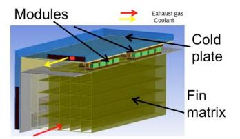
FIGURE 4. A cross-sectional view of the new TEG design concept for a passenger vehicle.
