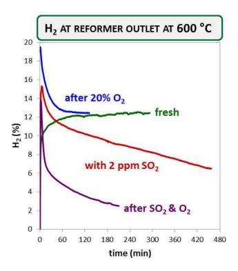
**FIGURE 5.** H<sub>2</sub> generation over the GTI catalyst for TCR as a function of time for the fresh catalyst, after exposure to  $O_2$ , in the presence of SO<sub>2</sub>, and after exposure to SO<sub>2</sub> followed by O<sub>2</sub>.
