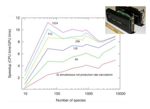
FIGURE 4. Speedup versus number of species in a chemical mechanism for calculations of combustion chemical kinetics on the GPU. Curves represent the number of reactors simultaneously solved on the GPU.
