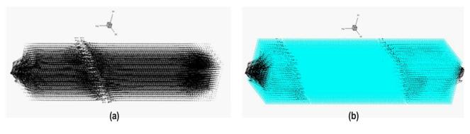
FIGURE 5. Square cylinders with moving piston showing velocity vectors and piston location in the grid. a) rectilinear motion of a slanted piston; b) rectilinear motion of two pistons moving simultaneously.
