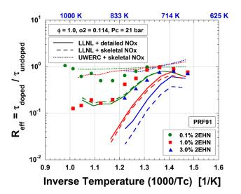
FIGURE 2. Effectiveness of 2EHN doped into a two-component gasoline surrogate, PRF91 at 21 bar and 11.4% oxygen.
