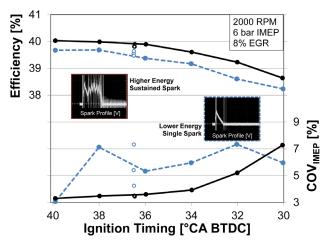
FIGURE 3. Combustion Stability and Indicated Thermal Efficiency for Two Distinct Spark Profiles Generated by the DEIS Ignition System
