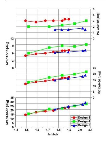
**FIGURE 4.** Pre-Chamber CA0-10, Main Chamber CA0-10, CA0-50, and CA10-90 vs.  $\lambda$ , 2,500 rpm , 47 kg/hr air flow – TJI Designs 3, 4, and 5
