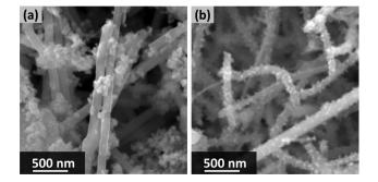
**FIGURE 3.** (a) Scanning electron micrograph of mixtures of unfunctionalized  $Zn_3P_2$  nanowires and copper nanoparticles. Here, nanowires and nanoparticles remained as individual units. (b) Scanning electron micrograph of copper nanoparticle decorated  $Zn_3P_2$  nanowires obtained by mixing BDT functionalized  $Zn_3P_2$  nanowires and copper nanoparticles.
