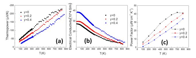
FIGURE 4. (a) Thermopower, (b) Electrical conductivity, and (c) Power factor of Mg<sub>2</sub>Si<sub>0.4</sub>Sn<sub>0.6-y</sub>Ge<sub>y</sub> (y=0, 0.2, 0.4) solid solutions with carrier concentration of (2.4±0.2)×10<sup>20</sup> cm<sup>-3</sup>.
