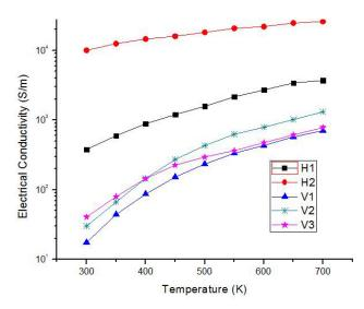
FIGURE 2. Electrical Conductivity of Mg<sub>2</sub>Si by VPS and Hot Press
