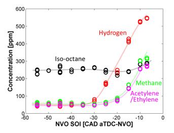
**FIGURE 4.** Select species concentrations determined by dump sampling and gas chromatography. Acetylene and ethylene are grouped due to inability of gas chromatograph columns to separate these  $C_{2}$  species.
