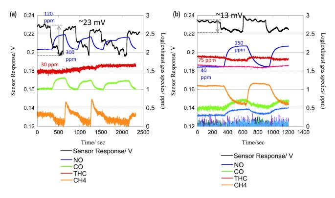
FIGURE 3. Sensor response at 0.2 μA bias to engine exhaust at a) 2,000 rpm and b) 1,600 rpm with EGR on and off. The NO, CO, THC and CH<sub>4</sub> concentration measured in the engine exhaust is also plotted.
