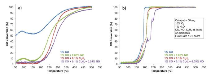
**FIGURE 2.** CO conversion as a function of temperature using a (a)  $AuCu/SiO_2$  or (b)  $Pt/Al_2O_3$  catalyst in the presence of 0.1%  $C_3H_6$ , 0.05% NO or 0.1%  $C_3H_6$  and 0.05% NO with a W/F = 0.25 g-h/mol. Catalysts were pretreated by calcination at 550°C for 16 h in 10%  $O_2$ , 1%  $H_2O$  and Ar (balance) at 75 sccm. Reaction conditions are in inset b.
