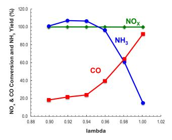
**FIGURE 2.** NOx and CO conversion and  $NH_3$  yield for the same data shown in Figure 1.
