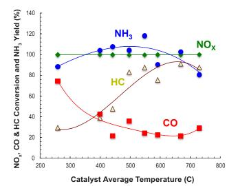
**FIGURE 3.** NOx, CO, and HC conversion and  $NH_3$  yield as a function of catalyst temperature over a broad range of engine speed and load combinations.
