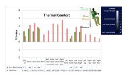
Thermal comfort computer-aided engineering tool validation results for one of the spot cooling test conditions. (Bozeman, General Motors)
