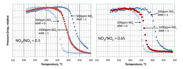
FIGURE 4. TPO studies with simulated exhaust presented as relative pressure drop versus temperature for NO<sub>2</sub>/NO<sub>x</sub> = 0.5 (left) and 0.65 (right), 150 g/L SCR catalyst loading, with SCR reaction (ANR=1) and without (ANR=0), 500 and 1,000 ppm NO<sub>y</sub>, 4 g/L initial soot loading, 35,000 GHSV.
