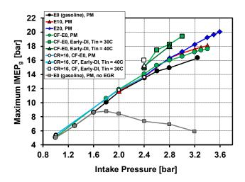
**FIGURE 5.** High-load limits as a function of intake pressure for premixed (PM) and Early-DI PFS fueling for several fuels. All data are for CR = 14:1, except those noted in the legend as CR =16, for which only CF-E0 was used. All points have no knock (RI  $\approx$ 5 MW/m<sup>2</sup>), and NOx and particulate emissions well below U.S. 2010 standards.
