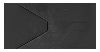
**FIGURE 3.** X-ray image through a steel injector nozzle showing bubbles that were drawn into the sac at the end of injection. The presence of these bubbles is likely to have an impact on emissions.
