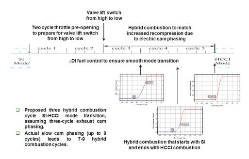
FIGURE 4. Proposed Hybrid Combustion Mode during the SI-HCCI Mode Transition
