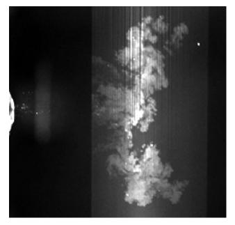
**FIGURE 5.** Raw planar Rayleigh scattering measurement. Molecular scattering from the ambient and the fuel jet is observable in the laser sheet area at the right.
