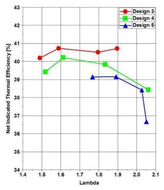
FIGURE 3. NTE vs.  $\lambda,$  2,500 rpm , 47 kg/hr air flow – TJI Designs 3, 4, and 5
