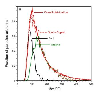
FIGURE 2. GCI particulate aerodynamic diameters under one low-load condition.
