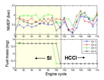
FIGURE 5. SI-HCCI Open-Loop Mode Switch—NMEP and Fuel Mass
