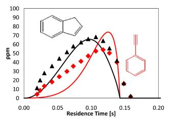
**FIGURE 2.** Comparison of simulations from the  $\alpha$ -methyl naphthalene chemical kinetic model with measurements [6] of intermediate species in a flow reactor for an equivalence ratio of 0.5 at 1 atm. The intermediate species shown are indene and phenylacetylene.
