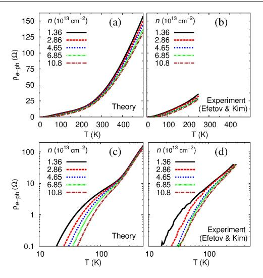
**FIGURE 5.** Electrical resistivity of n-doped graphene arising from electron-phonon interactions versus temperature incorporating electron-electron interaction effects [(a) and (c)] and the corresponding experimental data from Ref. [15] [(b) and (d)]. Quantities are plotted in linear scale in (a) and (b) and in logarithmic scale in (c) and (d).
