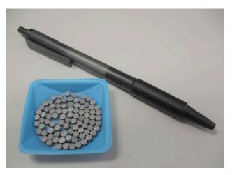
FIGURE 2. Sample MgSi TE material created with cold pressing and sintering. Production of elements at a rate of 3,000 pieces per hour was demonstrated.
