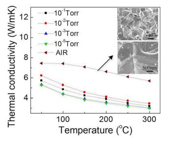
**FIGURE 5.** Thermal conductivity of layered ZnO materials sintered in vacuum compared with samples sintered in air. The layered structure strongly reduces thermal conductivity, while still allowing adequate electrical conductivity.
