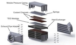
**FIGURE 5.** Exploded view of a detailed mechanical design of a TEG for a BFV.
