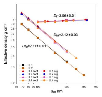
FIGURE 3. Plot of the calculated effective density as a function of mobility diameter for GCI particulates generated under low-load and high-load conditions.
