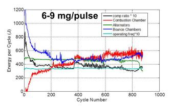
FIGURE 5. Energy Balance During Example Combustion Experiment
