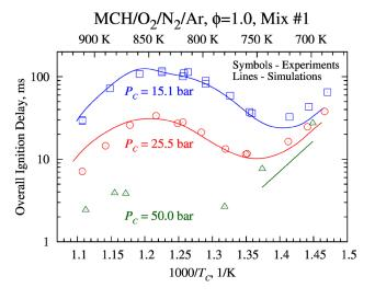
**FIGURE 3.** Comparison of the methylcyclohexane model with experimental ignition data from an RCM [5], for a stoichiometric mixture, over a range of temperatures, and at pressures of 15, 25 and 50 bar.
