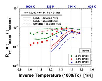
**FIGURE 3.** Effectiveness of 2EHN doped into a three-component gasoline surrogate, TRF91 at 21 bar and 11.4% oxygen.
