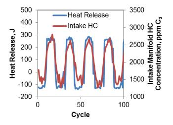
FIGURE 3. Time Series of Heat Release and Intake Hydrocarbon (HC) Concentration
