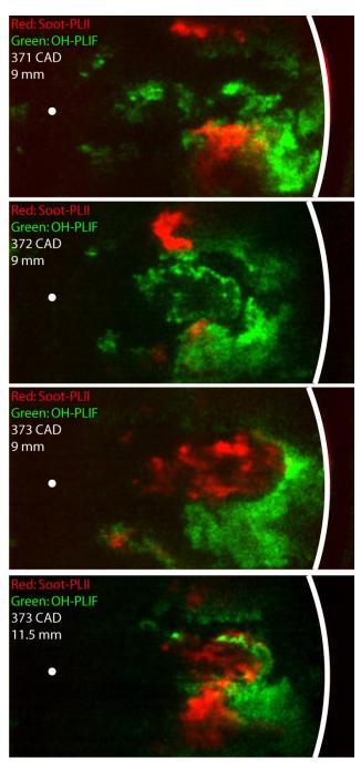
**FIGURE 4.** Instantaneous images of soot-PLII (red) and OH-PLIF (green) with laser sheets horizontal at elevations below the firedeck as indicated on the images. The soot-PLII and OH-PLIF are simultaneous in each image, but the images are from different cycles.
