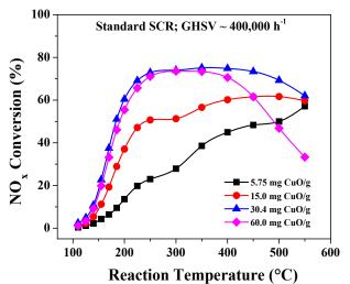
**FIGURE 5.** NOx NH<sub>3</sub> conversion as a function of temperature on Cu-SAPO-34-ACS samples formed by calcining xx mg CuO/1g SAPO-34 mixture at 800°C for 16 h. Standard SCR reactant feed contains 350 ppm NO, 350 ppm NH<sub>3</sub>, 14% O<sub>2</sub>, 2.5% H<sub>2</sub>O balanced with N<sub>2</sub>. Samples are denoted as 5.75 (**■**), 15.0 (**●**), 30.4 (**▲**) and 60.0 (**♦**) mg CuO/g, respectively. Gas hourly space velocity (GHSV) = 400,000 h<sup>-1</sup>.
