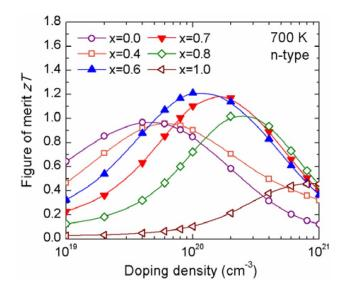
**FIGURE 6.** Calculated figure of merit *ZT* as a function of doping density for n-type  $Mg_2Si_{1,x}Sn_x$  with varying x=0~1.0 at 700 K. The lattice thermal conductivity is assumed to be 1.0 W/mK for all the compositions.
