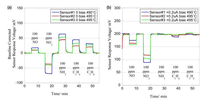
FIGURE 1. Comparison of the sensor response of three different mixed-potential sensors manufactured by ESL and operated under a) zero bias and b) 0.2 µA bias.
