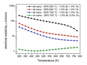
**FIGURE 3.** Electrical resistivity vs. temperature for Yb- and Bi-doped Mg<sub>2</sub>Si and the effect of grain size.
