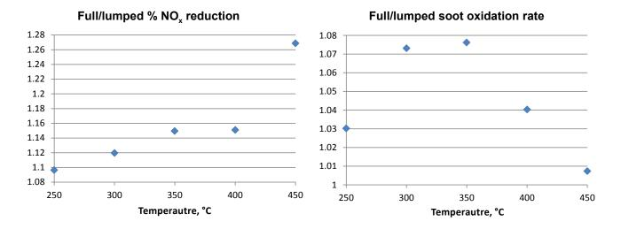
FIGURE 5. Ratio of full versus lumped SCRF model simulation as a function of temperature for NO<sub>x</sub> conversion (left) and soot oxidation (right), 150 g/L SCR catalyst loading, 500 ppm NO<sub>y</sub>, 4 g/L initial soot loading, NO<sub>2</sub>/NO<sub>x</sub> = 0.5, ANR = 1, 35,000 GHSV.
