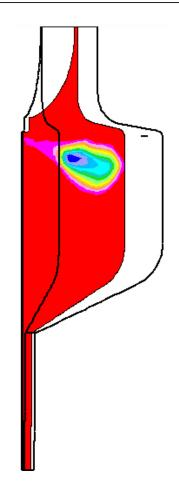
**FIGURE 1.** Temperature contour from transported PDF simulation of the ignition test in the Cetane ID 510. This is part of the model validation work. We perform high-speed optical imaging in the same apparatus.
