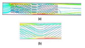
FIGURE 1. Representative plot of flow streamline visualization for louvered fins in exhaust gas heat exchanger.
