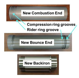
**FIGURE 4.** New Piston Design Incorporates Rider Rings and Thinner Compression Rings
