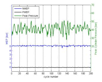
FIGURE 3. 200 Cycles of the IMEP and Peak In-Cylinder Pressure Signals
