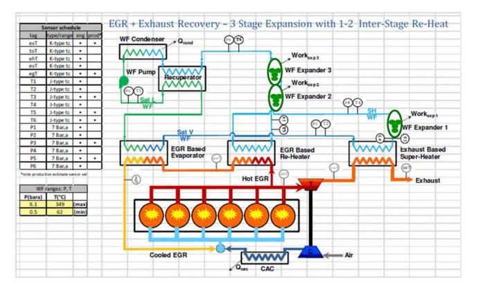
FIGURE 3. Architecture 4 - Rankine Cycle with Three-Stage Roots Expander
