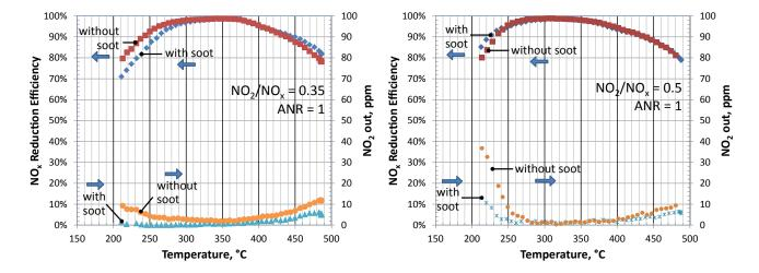
FIGURE 1. NO<sub>x</sub> reduction performance and post-filter NO<sub>2</sub> concentration with simulated exhaust versus temperature for NO<sub>2</sub>/ NO<sub>x</sub> = 0.35 (left) and 0.5 (right), 150 g/L SCR catalyst loading, with and without 4 g/L initial soot loading, 500 ppm NO<sub>x</sub>, ANR = 1, 35,000 gas hourly space velocity (GHSV).
