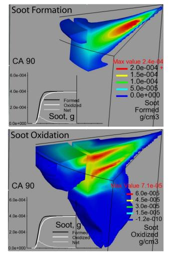
**FIGURE 5.** Time-integrated spatial distribution of soot formation (top) and soot oxidation (bottom) predicted by computer models.
