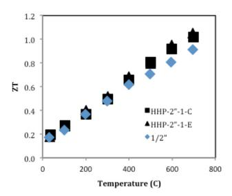
**FIGURE 1.** Comparison of ZT, a thermoelectric figure-of-merit, for a 2" hot-pressed disc sample of half-Heusler material with a  $\frac{1}{2}$ " baseline sample.
