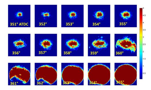
**FIGURE 5.** Sequence of SACI images from optical engine showing rapid transition from flame to autoignition. Average chemiluminescent intensity for E30 with SA at 40° before top-dead center and  $\Phi$ =0.45 at 700 RPM.
