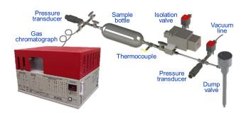
FIGURE 2. Schematic of dump valve, sample gas manifold, and gas chromatograph.
