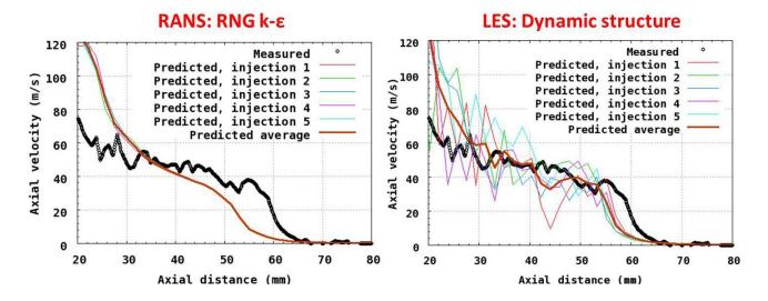
FIGURE 4. Axial velocity vs. axial distance compared between RANS RNG k-ε and LES dynamic structure models against experimental data from Meijer, et al. [7]. Multiple realizations show no cyclic variability with RANS, whereas significant shot-to-shot variations are captured with the LES model.
