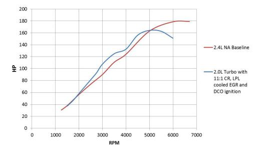
FIGURE 4. Horsepower of Phase 3 2.0-L Turbocharged Engine compared to Baseline
