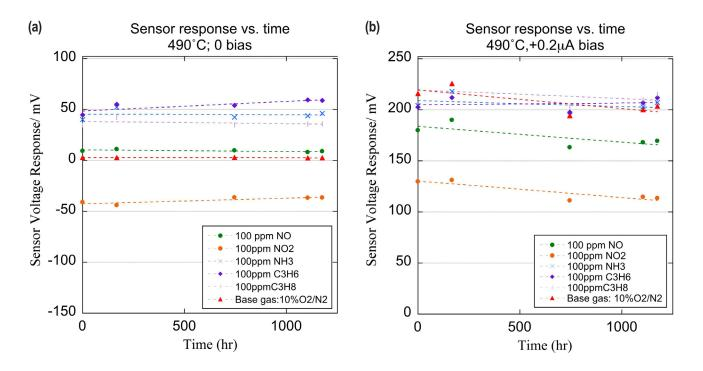
FIGURE 2. Stability of a mixed-potential sensor manufactured by ESL and operated E Inc.under a) 0.0 µA bias and b) 0.2 µA bias, for 1,000 hours.
