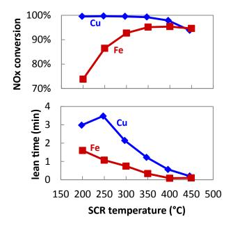
**FIGURE 5.** Comparison of Cu- and Fe-based performance on the bench flow reactor. In addition to higher NOx conversions obtained with the Cu SCR, longer lean periods were obtained thereby resulting in less fuel penalty.
