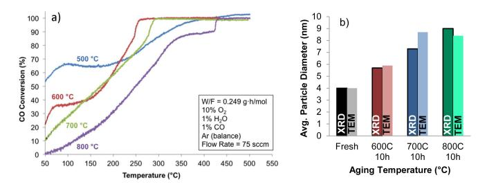
**FIGURE 4.** (a) CO conversion as a function of temperature after hydrothermal aging at 500, 600, 700 and 800°C for 10 h under 10%  $O_2$ , 1%  $H_2O$  and Ar. Reaction conditions: 1% CO, 1%  $H_2O$ , 10%  $O_2$  and Ar with a W/F = 0.5 g·h/mol at a flow rate of 75 sccm. (b) The size distribution histogram of metallic particles on AuCu/SiO<sub>2</sub> after thermal aging.
