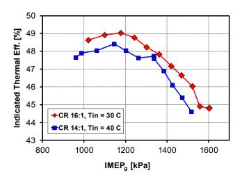
**FIGURE 4.** Comparison of TEs for CR = 16:1 and CR = 14:1 as a function of IMEP<sub>g</sub> for Early-DI PFS fueling at  $P_{in}$  = 2.4 bar and RI ≈5 MW/m<sup>2</sup>.  $T_{in}$  = 30 or 40°C as noted in the legend.
