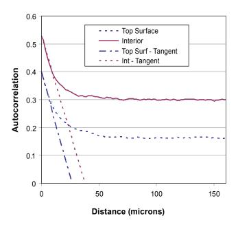
**FIGURE 6.** Autocorrelation plots for the void phase at the top surface and in the interior of a cordierite filter wall.
