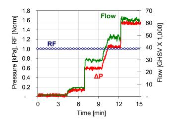
**FIGURE 5.** Effect of increasing exhaust flow rate through the DPF on pressure drop and RF signal response, showing the RF signal to be unaffected by variations in exhaust flow.
