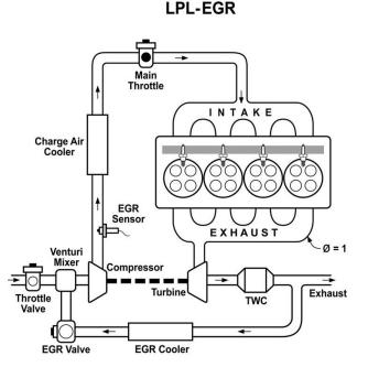
FIGURE 1. LPL EGR System Applied to Turbocharged Engine
