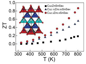
**FIGURE 4.** ZT vs. temperature for  $Cu_{2\kappa_x}Zn_{1,x}SnSe_4$  (0  $\leq x \leq$  0.2) and crystal structure of stannite compositions  $Cu_2ZnSnSe_4$ .
