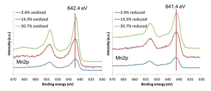
FIGURE 4. XPS spectra for the MnO<sub>x</sub>/CeO<sub>2</sub> catalysts prepared by incipient wetness impregnation after oxidation (left) and after reduction (right) in air and H<sub>2</sub>, respectively, at 500°C for one hour.
