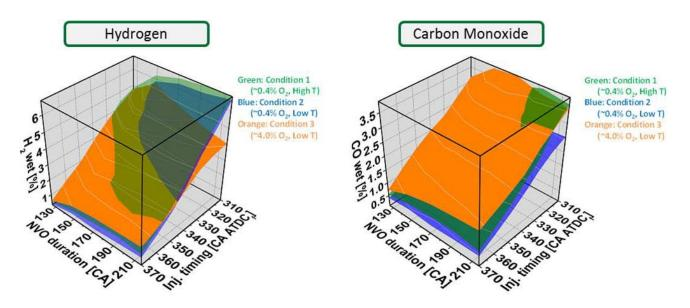
FIGURE 2. Experimental response surfaces of H<sub>2</sub> and CO as a function of NVO duration and fuel injection timing.
