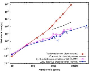
**FIGURE 3.** The computational cost of the adaptive preconditioner technique shows near linear scaling for new molecules and mechanism classes. Examples include: (a) methylcyclohexane (1,000 species [10]); (b) 3-component biodiesel surrogate (3,300 species [11]); and (c) and an automatically generated mechanism for hydrocarbons up to C9 (39,000 species [12]).
