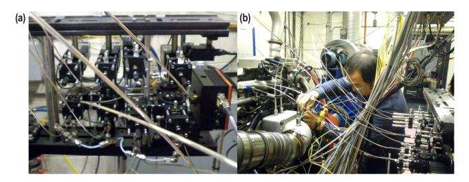
FIGURE 1. Multiplex laser-based EGR probe instrument (a, left) and EGR probe installation in the engine (b, right).
