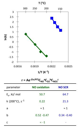
FIGURE 3. Arrhenius plot and power law rate expression parameters for NO oxidation and NO SCR over a commercial copper-exchanged small-pore zeolite.
