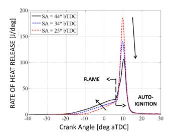
**FIGURE 7.** KIVA-CFMZ model predicted rate of heat release for three SACI cases. Advancing the spark timing and decreasing NVO with fixed CA50 increases the fraction of flame heat release and significantly reduces the peak rate of heat release during compression ignition.
