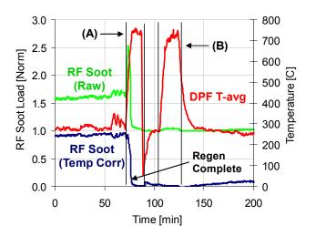
**FIGURE 6.** Vehicle data from a heavy-duty truck showing rapid soot oxidation during high temperature regenerations and potential for regeneration fuel savings of 50% to 75% through accurate measurement of DPF soot levels using RF sensing.
