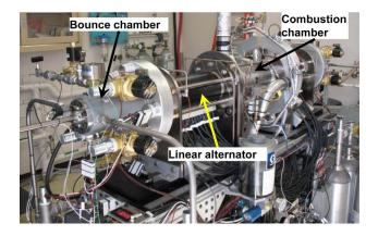
FIGURE 1. Sandia FPEG Research Prototype
