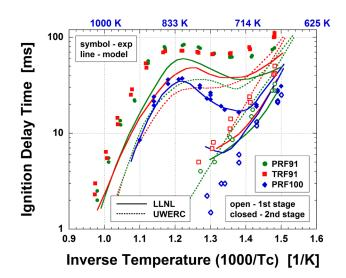
**FIGURE 1.** Ignition delay times as function of temperature for three undoped fuels, PRF91, TRF91 and PRF100 at 21 bar and stoichiometric conditions; PRF91 and TRF91 conducted at 11.4% oxygen, PRF100 at 21% oxygen.
