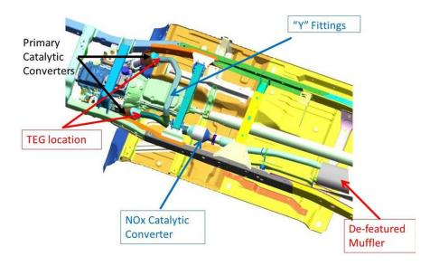
**FIGURE 1.** Schematic view of the underside of the full size pickup showing the proposed location of the dual TEG subunits and other features of the exhaust system.
