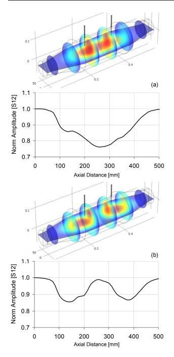
FIGURE 1. Comparison of simulation results with experiments showing predicted and experimentally-verified electric field distributions for first (a) and second (b) resonant modes. Electric field distribution corresponds to spatial resolution of the measurement.
