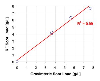
FIGURE 3. Comparison of RF and gravimetric measurements of DPF soot load up to 8 g/L.
