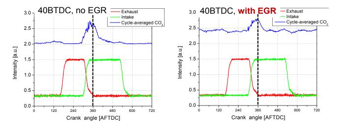
FIGURE 5. EGR probe residual backflow measurements with intake-exhaust valve overlap centered at 40° BTDC and with and without external EGR; the vertical black dashed line indicates TDC.
