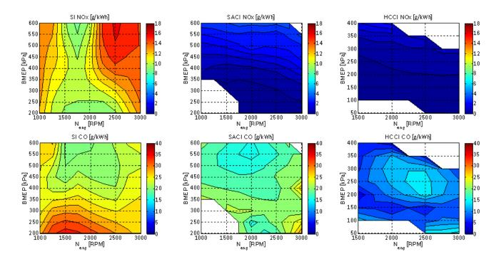
FIGURE 3. NOx and CO Engine-Out Emission Performance under Combustion Modes of SI, HCCI, and SACI Observed on the ACCESS Prototype I Engine
