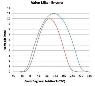
FIGURE 3. VVA Atkinson and Otto Cycle Cam Lift Profiles
