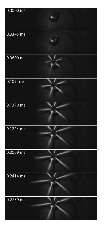
**FIGURE 6.** Spray injection of n-heptane in the combustion chamber of a PAC Cetane ID 510. Images captured at 29,000 frames per second with a Phantom v7.1 monochrome camera.
