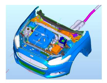
FIGURE 5. CAD Powertrain as Installed in Vehicle
