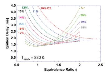
**FIGURE 4.** Variation of ignition delay with  $\varphi$  and  $O_2$  at a fixed ambient temperature of 880 K.
