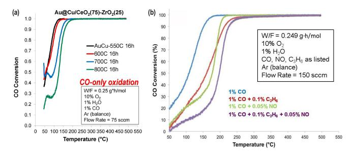
FIGURE 5. Supporting AuCu on a ceria/zirconia support showed improved durability to (a) thermal effects and (b) in the presence of NO/HCs.
