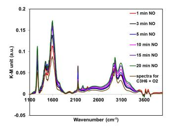
**FIGURE 2.** Emergence of new peak upon exposure to 500 ppm NO after 45 minutes of exposure to 500 ppm  $C_3H_6$  at 380°C (500 ppm  $C_3H_6$ , 500 ppm NO, 1% O<sub>2</sub>, balanced by He).
