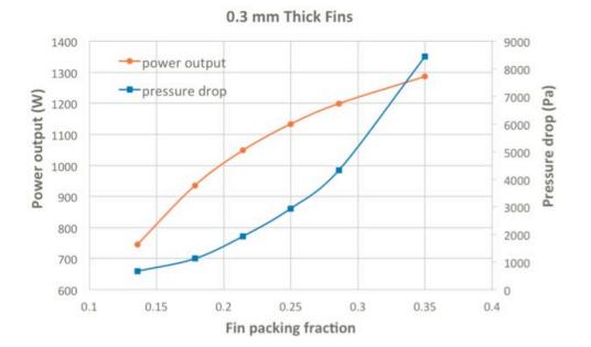
FIGURE 6. Electrical power output and pressure drop of the TEG shown in Figure 5 as a function of fin packing fraction for a fin thickness of 0.3 mm.
