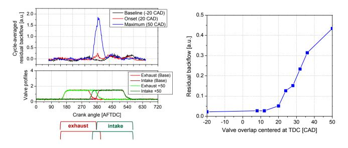
FIGURE 6. EGR probe residual backflow measurements with increasing intake-exhaust valve overlap approximately centered at TDC.
