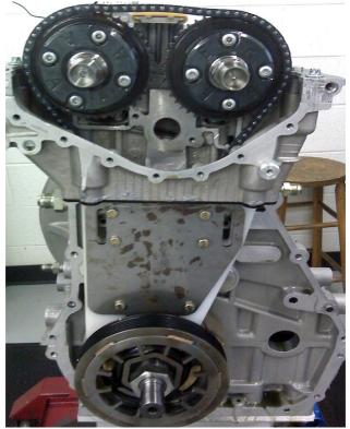
FIGURE 7. VCR Engine Timing Chain System
