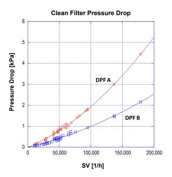
FIGURE 2. Clean filter pressure drops of two different filters.
