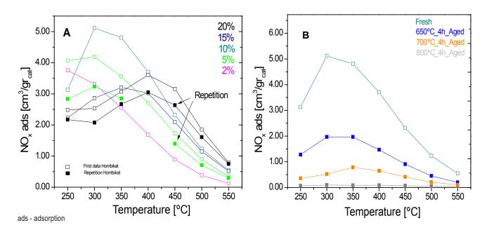
FIGURE 1. Panel A: Amounts of stored NOx during NOx storage tests on fresh Pt(1)K(x)/TiO2, K = 2, 5, 10, 15, 20 w/w%. Panel B: NOx stored amounts during NOx storage tests on fresh and aged (at 650°C, 700°C and 800°C for 4 h) Pt(1)K(10)/TiO<sub>2</sub>.
