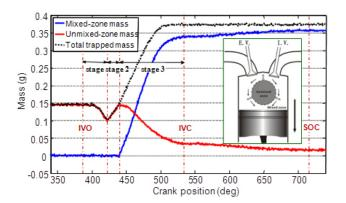
FIGURE 1. Simulated Charge Mixing Responses of the Turbulence-Based Model
