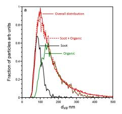
Gasoline compression ignition particulate aerodynamic diameters under one low-load condition. (Stewart, PNNL)
