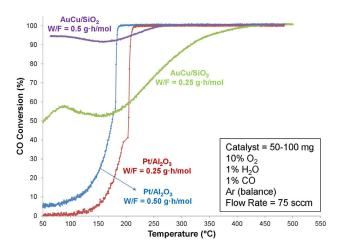
**FIGURE 1.** CO conversion, with different weight to flow ratios (W/F), as a function of reaction temperature for AuCu/SiO<sub>2</sub> and Pt/Al<sub>2</sub>O<sub>3</sub>. Catalysts were pretreated by calcination at 550°C for 16 h in 10% O<sub>2</sub>, 1% H<sub>2</sub>O and Ar (balance) at 75 sccm. Reaction conditions are in inset of the figure.
