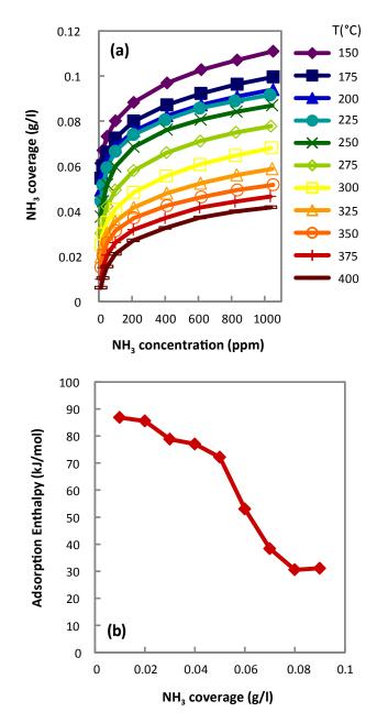
**FIGURE 4.** (a) Equilibrium  $NH_3$  storage isotherms and (b)  $NH_3$  adsorption enthalpy as a function of  $NH_3$  coverage over a commercial copperexchanged small-pore zeolite.
