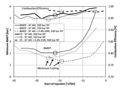
FIGURE 1. Minimum Fueling Rates for 500 bar and 250 bar Injection Pressure
