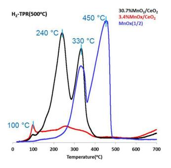
**FIGURE 3.** Temperature programmed reduction for 3.4 and 30.7%  $MnO_x/CeO_2$  prepared by incipient wetness impregnation compared with pure MnOx. All samples were calcined at 500°C for one hour prior to the temperature programmed reduction measurements.
