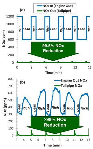
**FIGURE 4.** Experimental results from bench reactor (a) and engine (b) studies showing the combined performance of a TWC+SCR system. Tailpipe emission levels are also shown in Table 1.
