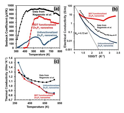
**FIGURE 2.** Plots showing the variation of (a) Seebeck coefficients, (b) electrical conductivities, and (c) thermal conductivities of both a functionalized and unfunctionalized  $Zn_3P_2$  nanowire pellet with temperature. For comparison, thermoelectric properties of  $Zn_3P_2$  microparticles previously reported by Nagamoto *et al.* are also included.
