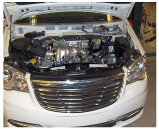
FIGURE 5. Alpha 2 Multi-Air Multi-Fuel Engine in Vehicle
