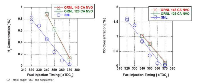
FIGURE 3. Comparison of ORNL and SNL experimental measurements of H<sub>2</sub> and CO generation as a function of fuel injection timing at comparable engine operating conditions.
