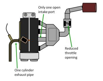
FIGURE 2. Reconfigured Single-Cylinder Metal Engine Diagram
