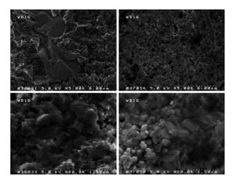
**FIGURE 1.** SEM images of the methanol-etched fracture faces of 1.0% Yb doped  $Mg_2Si$ . The two left images show the microstructure of a sample sintered at 500°C using 5k (top left) and 20k (bottom left) magnification. The images on the right were taken on a sample sintered at 650°C. The top right one at a magnification of 5k, the bottom right one at 20k.
