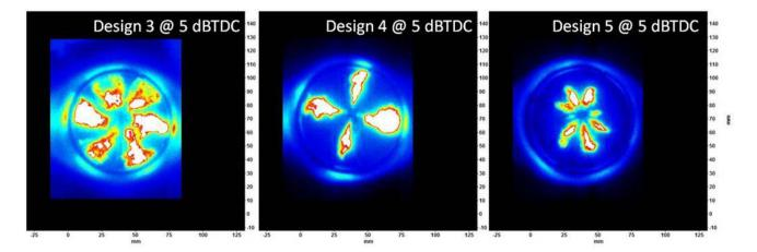
FIGURE 6. Optical Data @ 5 degrees before top-dead center (dBTDC) - TJI Designs 3, 4, and 5
