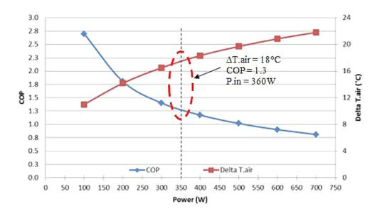
FIGURE 4. Calorimeter Performance and Efficiency of TE Device in Heating Mode
