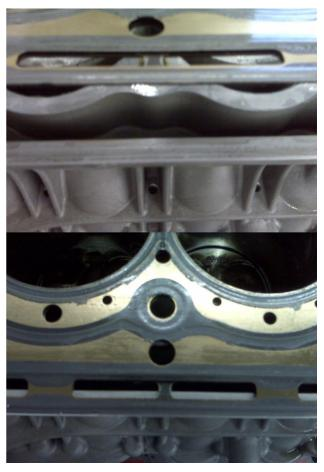
FIGURE 4. Internal EGR Passage Mismatch between ENVERA Block and OEM Head Gasket
