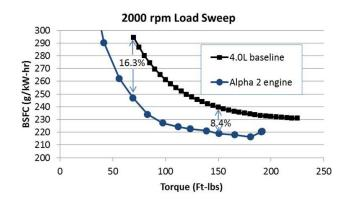
FIGURE 1. 2,000 RPM Load Sweep
