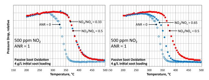
FIGURE 3. TPO studies with simulated exhaust presented as relative pressure drop versus temperature for NO<sub>2</sub>/NO<sub>x</sub> = 0.33 and 0.5 (left) and 0.5 and 0.65 (right), 150 g/L SCR catalyst loading, with SCR reaction (ANR=1) and without (ANR=0), 500 ppm NO<sub>x</sub>, 4 g/L initial soot loading, 35,000 GHSV.
