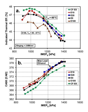
**FIGURE 2.** Gross indicated thermal efficiency (2a), and CA50 (2b) as a function of IMEP<sub>g</sub> at P<sub>in</sub> = 2.4 bar, RI ≈5 MW/m<sup>2</sup>, 1,200 rpm, and T<sub>in</sub> = 60°C except for E100, for which T<sub>in</sub> varied from 95-87°C as load was increased.
