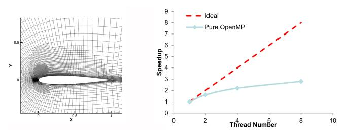
**FIGURE 2.** Transonic flow over a 3-D National Advisory Committee for Aeronautics 0012 airfoil at 4° angle of attack using hp-adaptive PCS FEM. a) adapted final grid; b) OpenMp speed-up as central processing units are increased (threading).
