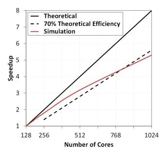
**FIGURE 5.** Speedup calculations for a typical internal combustion engine simulation run on 128-1,024 cores on a high-performance computing cluster at Argonne National Laboratory. Linear (ideal) speedup curve is also shown.
