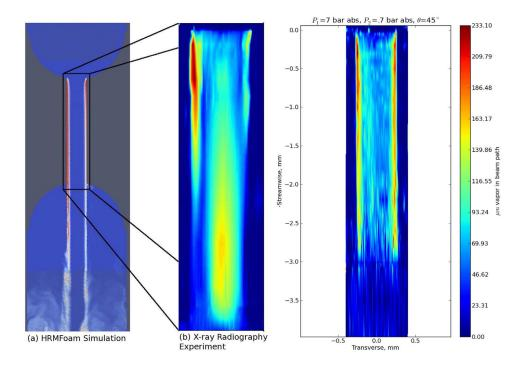
**FIGURE 2.** Simulations of cavitating flow (left) are compared to X-ray radiography measurements done in 2012 (middle) and 2013 (right). The newest measurements show much better symmetry, with cavitation only along the walls of the nozzle as expected. The improved measurements are being used for flow model development and validation.
