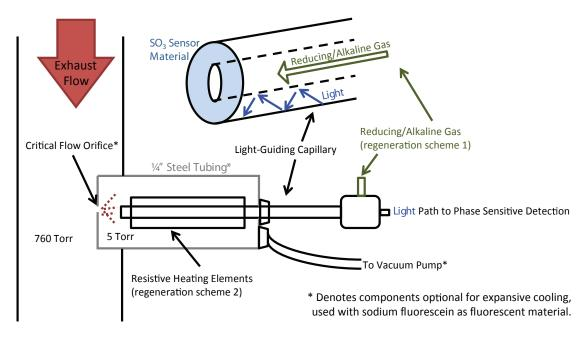
**FIGURE 1.** The probe concept can exploit expansive cooling from atmospheric to near-vacuum pressure, and a light-guiding capillary allows the sol gel containing a material, copper zeolite, sensitive to SO<sub>3</sub> and to be interrogated with laser induced luminescence and regenerated with an alkaline gas.
