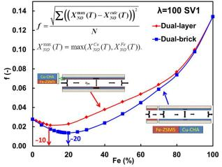
**FIGURE 3.** Compositional optimization of the dual-layer and brick Fe-Cu SCR catalysts.
