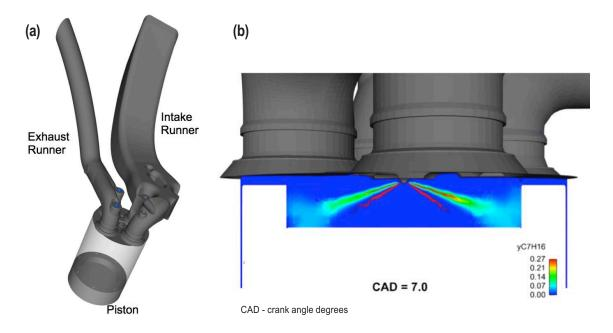
**FIGURE 5.** (a) Geometry of the flow domain analyzed for the Sandia Heavy Duty Fuels engine, and (b) fuel distribution at 7 degrees after top-dead center for conventional diesel operation using n-heptane as a kinetic surrogate.
