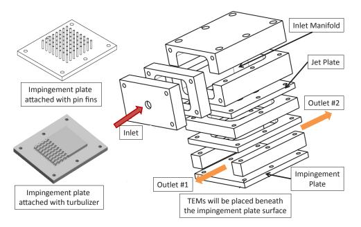
**FIGURE 4.** Schematic of test shroud based on jet impingement heat transfer mechanism. Flexible design enables evaluation of various surface enhancements such as pin fins and turbulizer.
