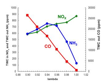
**FIGURE 1.** NOx at the TWC inlet position and CO and  $NH_3$  at the TWC outlet position as a function of equivalence ratio.
