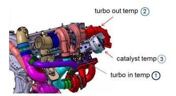
FIGURE 2. Cold-Start Catalyst Temperature Engine-Only Surrogate Test Setup
