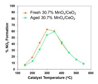
**FIGURE 1.** Effect of aging on the activity of 30.7% MnO<sub>x</sub>/CeO<sub>2</sub> catalyst prepared by incipient wetness impregnation. Aging was performed in 10% steam in air at 700°C for one hour. Reaction conditions: 50 mg catalyst, 156 sccm total flowrate, gas composition: 200 ppm NO, 10% O<sub>2</sub>, 10% steam, balance N<sub>2</sub>.
