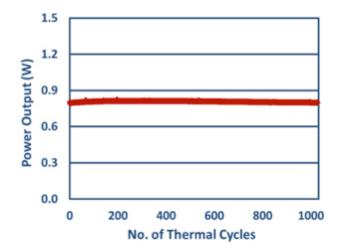
**FIGURE 2**. Power output of a thermoelectric device thermally cycled between 600°C and 100°C. The device shows <1% degradation in performance over 1,000 cycles.
