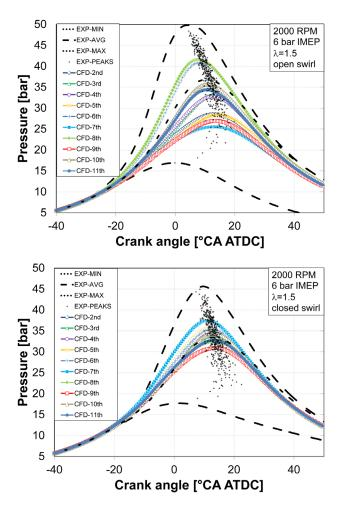
FIGURE 4. Experimental and Numerical Cyclic Variability for Two Intake Flow Configurations at 2,000 RPM, 6 bar IMEP, and  $\lambda{=}1.5$
