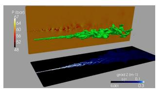
**FIGURE 2.** Instantaneous structure of the Spray-A case at 0.27 ms, which is the point of injection just prior to auto-ignition. The green iso-contour represents the mass fraction of n-dodecane at a value of 0.5. Also shown are the instantaneous pressure and scalar dissipation fields along the center plane of the jet.
