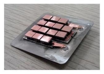
FIGURE 3. High-temperature thermoelectric module with the hot-side casing removed.
