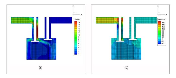
FIGURE 4. Flow in 2-valve engine simulation using hp-adaptive PCS FEM system. Velocity magnitude on center slice (a) and pressure on center slice (b).
