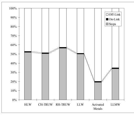
Figure 4.10. Distribution of the Total Incident-Free Dose to Members of the Public, Persons at Stops, and Off-link and On-link Receptors for all Cargo Types, from the Waste Management Programmatic EIS, Rail Transport (DOE, 1997b)
