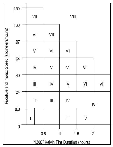
Figure 6.9. Scheme for NUREG-0170 Classification by Accident Severity Category for Rail Accidents (Source: NRC 1977a)
