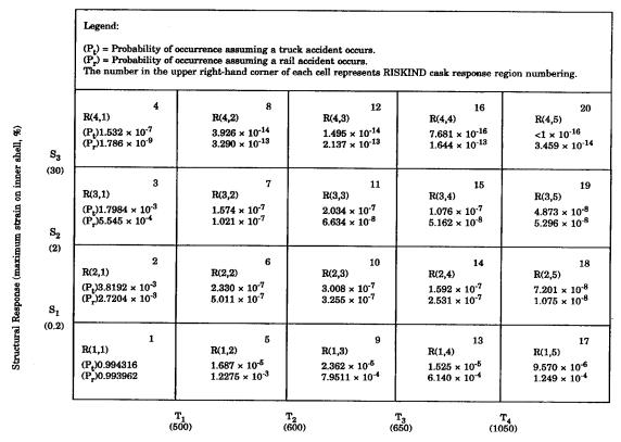
Thermal Response (lead midlayer thickness temperature, °F)
