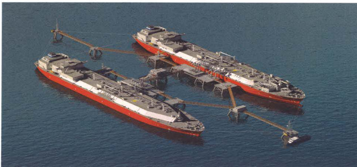
Figure 4D: Aguirre Offshore GasPort with FSRU and LNGC
