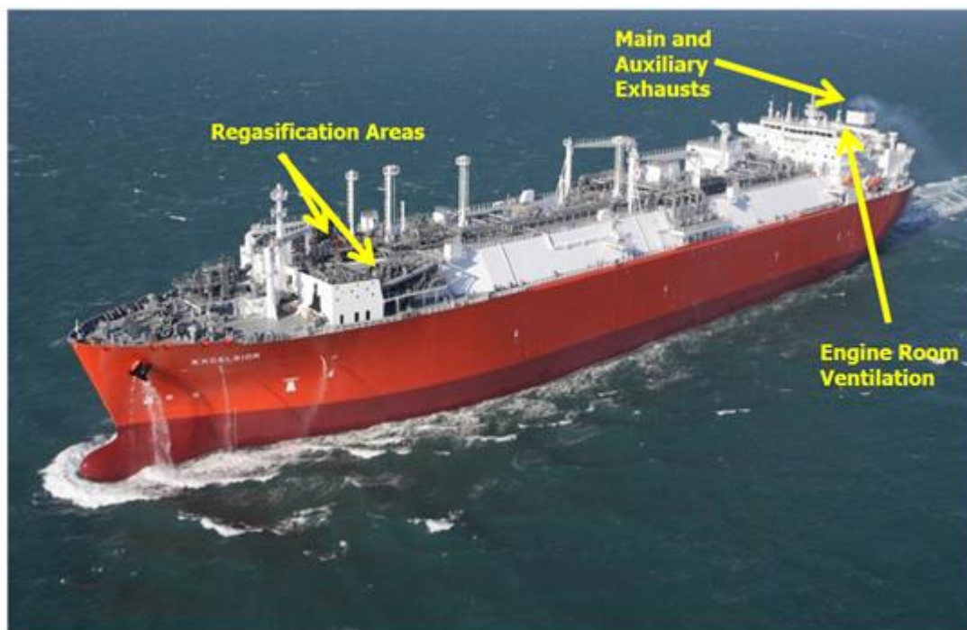
Figure 4.10.2-2: Prototype EBRV Excelsior and Areas of Principal Sound Emission
