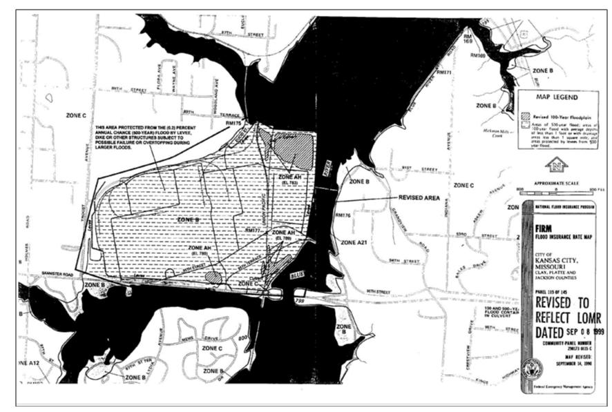
Figure 3-11. Applicable Flood Insurance Rate Map (annotated with modifications in the flood zones around the BFC) (Source: FEMA 1999)
