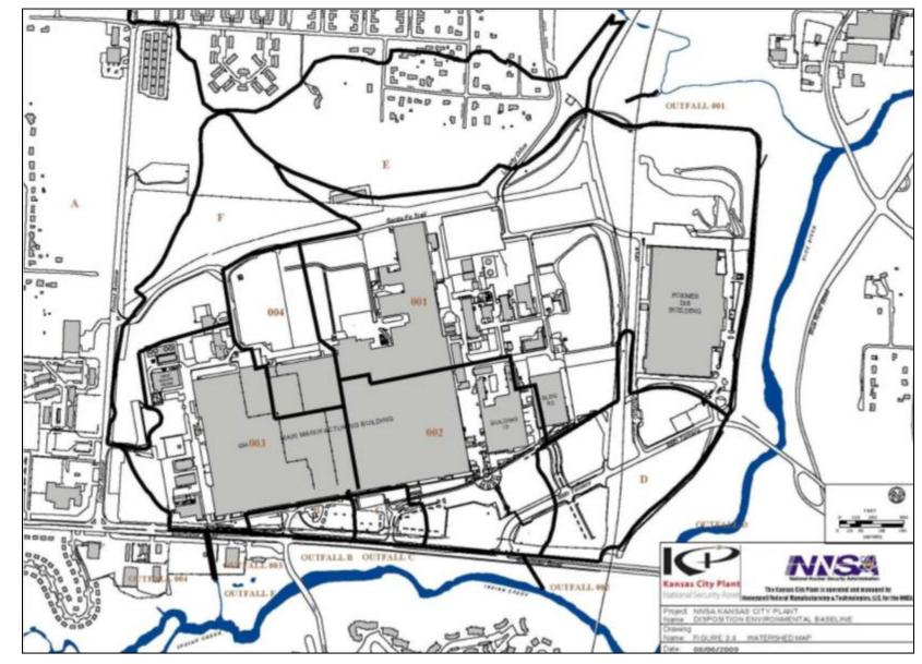
Figure 3-8. Drainage Areas on the BFC and the Outfalls to which They Drain (Source: Honeywell 2013)
