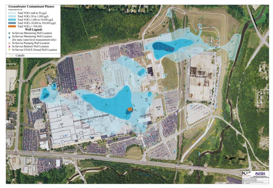
Figure 3-10. Volatile Organic Compound Contamination Plumes in Groundwater Beneath the BFC (Source: DOE 2012a)
