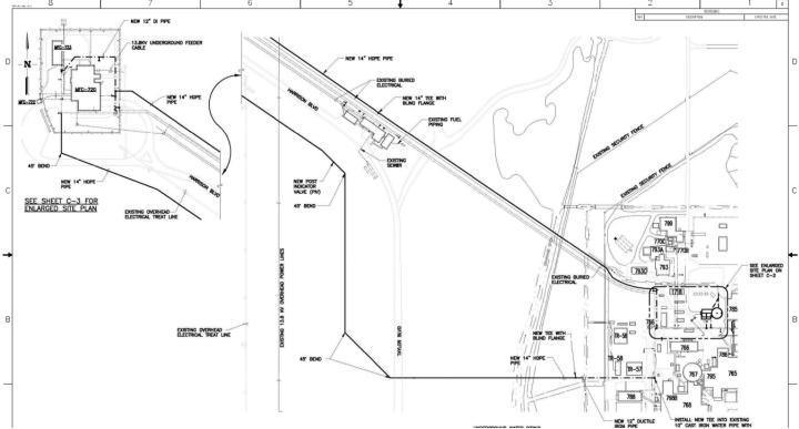
The fire/potable water system would be considered a Public Water, Non-Transient/Non-Community system and would disinfect, store, and pump fire and potable water from two existing wells to the existing MFC underground piping system. Water softening would be done at the point of use as required. Water softener regeneration water would be routed to the existing storm water system. New fire hydrants, sectional valves, and tees would be installed in the HDPE piping.
