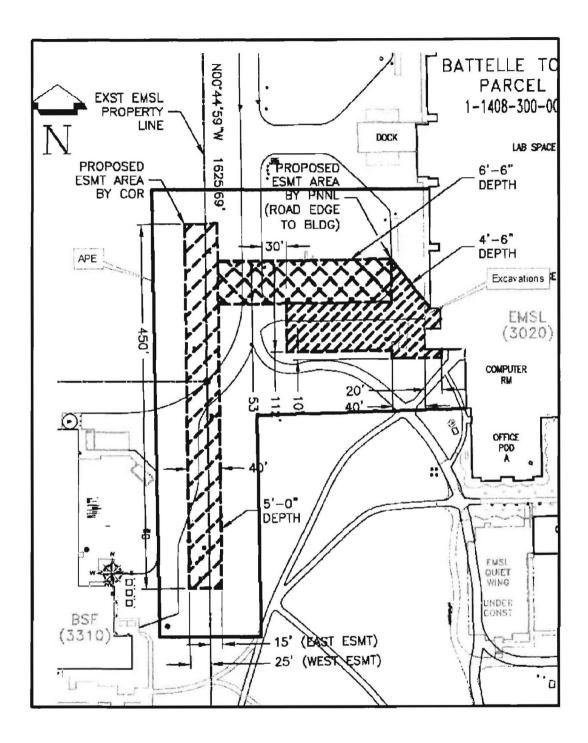
Figure 1. Engineer's drawing of project area with proposed excavations illustrated in diagonal hatch-marks
