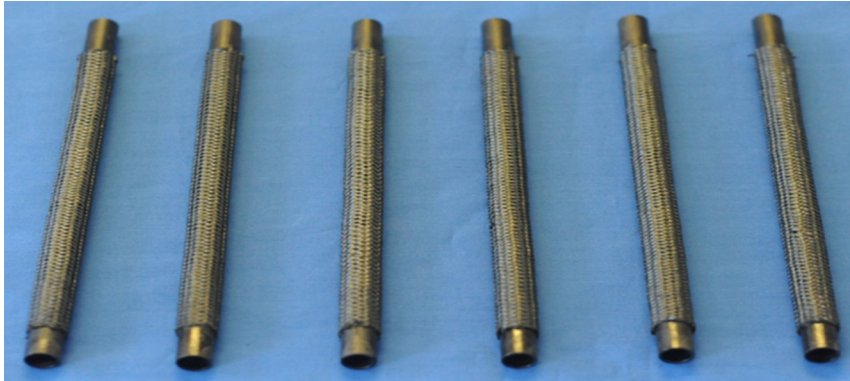
Figure 2: SiC CMC fuel rod cladding with metal liner
