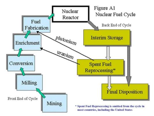
\*\*Note that the recycled uranium may be enriched as precursor to fuel fabrication. Also, transuranic (TRU) waste (with long-lived actinides) would likely be part of the stream for fuel fabrication to enable their burn-up in reactor.
