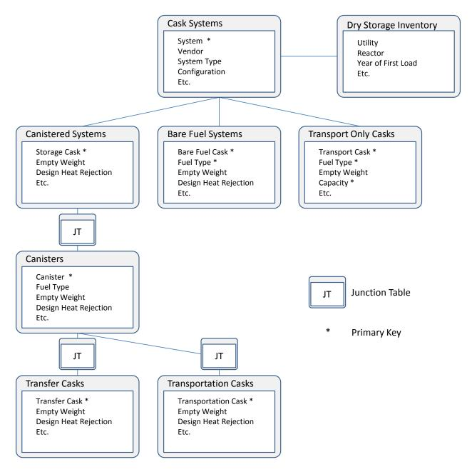
Figure 3.2-1 Dry Storage Cask/Inventory Database Structure
