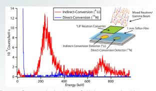
Figure 2. Spectra obtained from GaN detector using Li-6 indirect-conversion material (red) and direct-conversion of neutrons from N-14 (blue). Inset is a schematic of the experiment setup.
