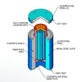
Figure 3. A cutaway illustration of the Holtec International, Inc. Hi-Storm 100 storage system. Once installed on a storage pad, these systems provide radiation shielding protection for the UNF and a barrier against intrusion.
