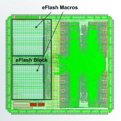
Figure 2. Application-specific integrated circuit test die.
