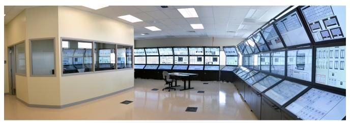
Figure 1. The virtual simulator at the Human Systems Simulation Laboratory.
