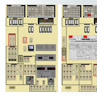
Figure 3. Example of legacy turbine control system computer (left) updated with a turbine HSI (right) on the glasstop panels of the Human Systems Simulation Laboratory.
