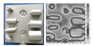
Figure 9. Joyo-pin target sample and intensity image of the target sample at  $177^{\circ}C$  and FD = 25.4 mm.
