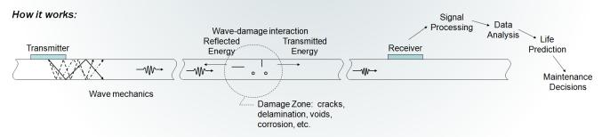
Diagram shows the through-transmission method; the pulse-echo method is similar but based on reflected energy.
