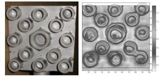
Figure 7. Fuel-pin target sample and intensity image of the target sample at  $177^{\circ}$ C and FD = 25.4 mm.
