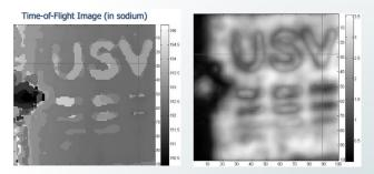
Figure 6. TOF (left) and intensity (right) images of the USV target sample at 177°C and FD = 25.4 mm.
