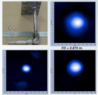
FD = 1.0 in. FD = 1.125 in. Figure 10. Ball-bearing target sample and beam diameter.
