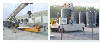
Figure 1. A horizontal dry storage system, (left image) and vertical dry storage system (right image). Both of these systems use welded stainless steel canisters to contain the UNF.
