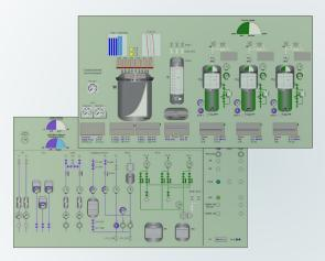
Figure 4. Advanced overview displays to aid operator monitoring and troubleshooting.
