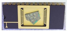
Figure 1. Photograph of several detectors fabricated on a GaN wafer, mounted in a standard dual inline package for testing.
