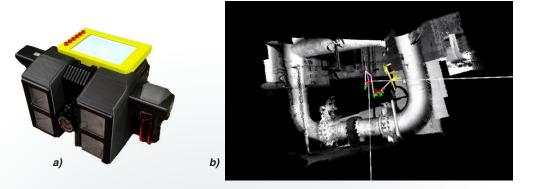
Figure 2. Phase II handheld 3D video camera (a) will be coupled with optimized registration software to create near real-time as-build models of large plant areas. Preliminary testing with DotProduct's Phi3D software created a registered point cloud (b) in less time than it took to take the data (4 sec registration for 10 sec of data).
