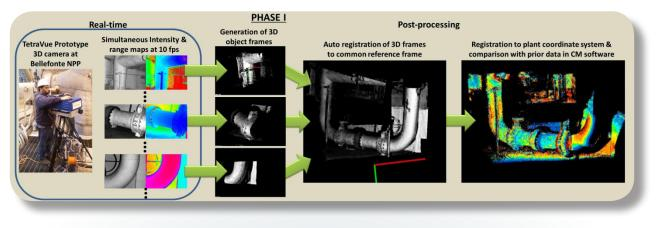
Figure 1. Phase I has demonstrated path to collect frames of intensity and range maps, convert to 3D frames, register these frames together, and then compare with design or prior as-built information in an NPP. This demonstration will be made robust and practical in Phase II.
