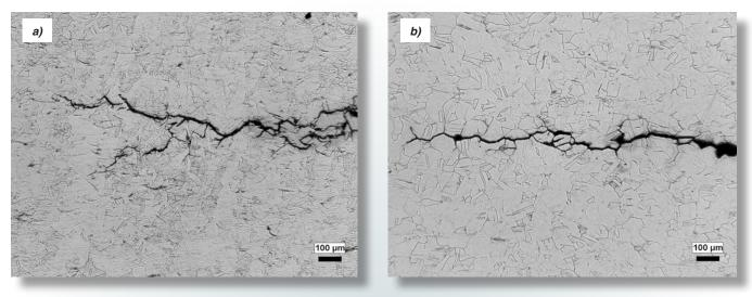
Figure 2. Cross-sectional image of stress corrosion crack on DMLM316L stainless steel after SCC test.
