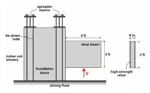
Figure 3. Preliminary elevation (left) and cross-section (right) views of deep beam specimens
