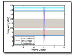
Figure 3. Dispersion curve of unit cell suppressed in the vertical direction.
