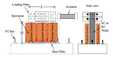
Figure 2. Test setup for conducting accident thermal plus lateral loading tests.
