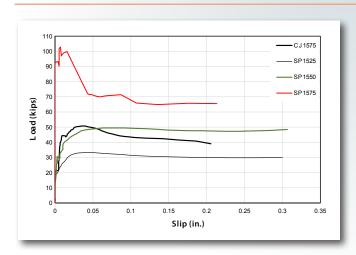
Figure 3. Load versus slip relationship for four different specimen configurations and tested as shown in Figure 2. Specimen CJ1575 (solid line) is a baseline specimen that is reinforced with internal concrete reinforcement. SP1525, SP1550, and SP1575 represent steel plate composite specimens with 0.25%, 0.50%, and 0.75% external reinforcement.
