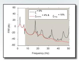
Figure 5. Attenuation zones of Unit Cell 3.
