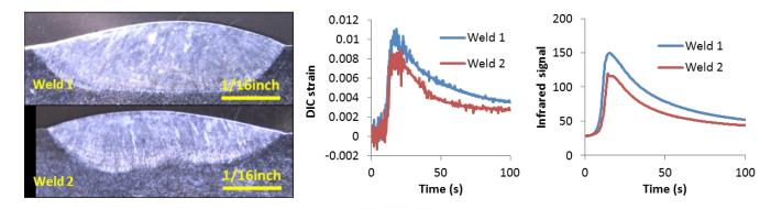
Figure 2. Variation of in-situ strain and IR signals positively correlates to a certain weld defect (Weld 1 - normal size; Weld 2 - undersize).
