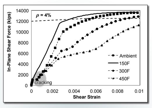
Figure 3. Effects of accident thermal loading on the in-plane shear behavior of SC walls.
