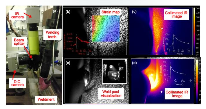
Figure 1. Integrated optical sensing technology for welding in-situ monitoring.
