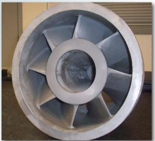
Figure 2: ALWR steam separator inlet swirler.
