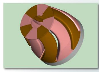
Figure 3. ALWR steam separator inlet swirler model.
