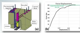
Figure 5: Direct shear test – (a) test setup and (b) applied force – displacement response
