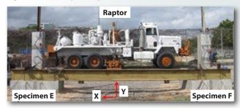
Figure 4: Test setup of 3D periodic foundation
