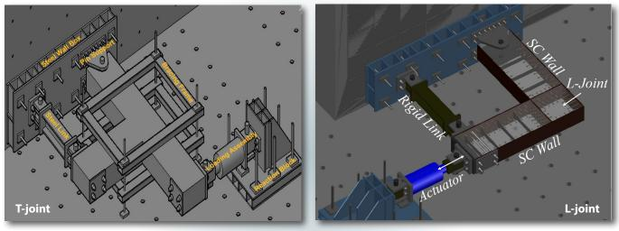
Figure 2: SC wall to wall connection test setup
