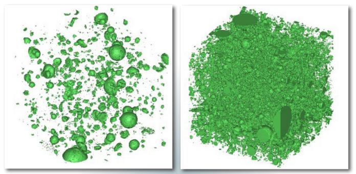
Figure 2: Reconstructed 3D images of pore structure (in green color) for UHPC (left) and conventional concrete (right)
