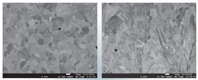
Figure 4: Micrographs showing microstructure/grain size between Inconel bar stock (left) and additively manufactured sample (right).
