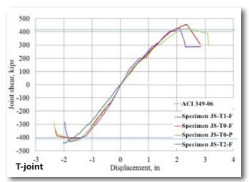
Figure 3: Joint shear – displacement responses
