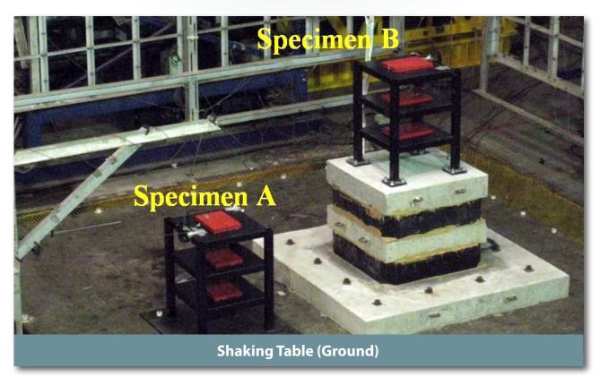
Figure 1: Test setup of 1D periodic foundation
