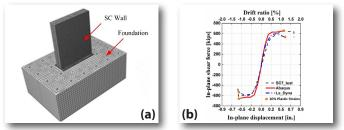
Figure 7: (a) In-plane shear analytical model test and (b) Analytically predicted response
