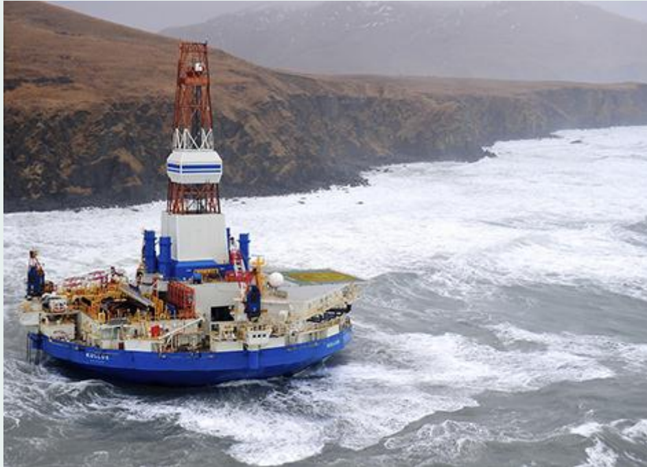
Figure 2-12. The drilling rig Kulluk aground on the shore of Sitkalidak Island in 2013. In this picture, the rig is weathering 40 mph winds and 20-foot seas as it waits to be recovered.
