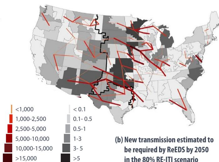
**Figure 3.** Existing transmission (a) and potential 2050 transmission (b).
