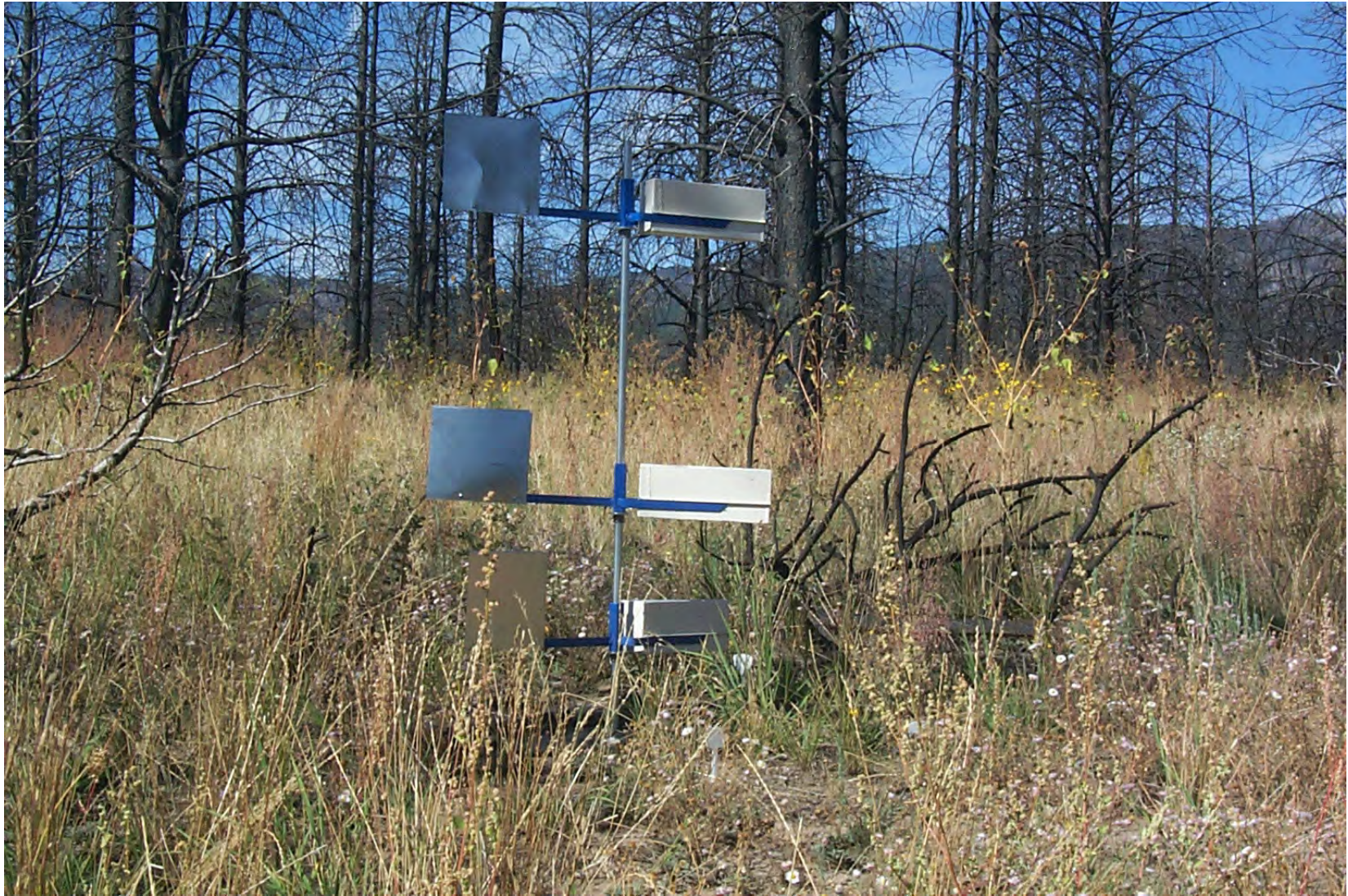
Figure 3 Field Dust Collector with Rotating Samplers at Three Heights
