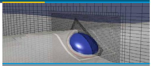
Computational fluid dynamics simulation of a WEC in focused waves.
