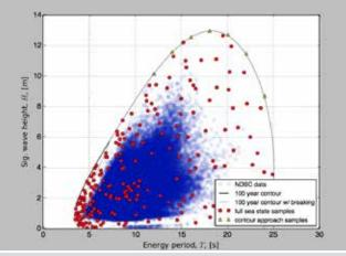
Analysis of National Data Buoy Center (NDBC) wave data to give 100-year return contour and sampling of sea states for survival analysis performed with <u>WEC</u> <u>Design Response Toolbox (WDRT).</u>
